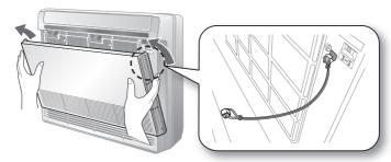
2. Grab the handle and slightly press the air filter down to bent the air filter. Then, pull the Air filter towards you and lift it up to remove the Air filter.
