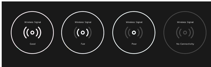
Figure 24. Wireless Extender Signal Strength Indicators
