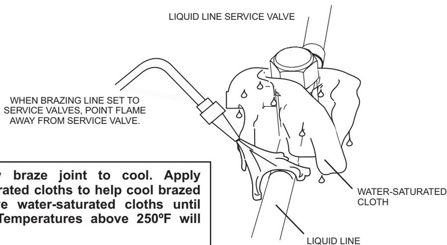
**IMPORTANT — Allow braze joint to cool. Apply additional water-saturated cloths to help cool brazed joint. Do not remove water-saturated cloths until piping has cooled. Temperatures above 250°F will damage valve seals.**
