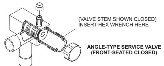
When service valve is **CLOSED**, the service port is open to the line set and indoor unit.
