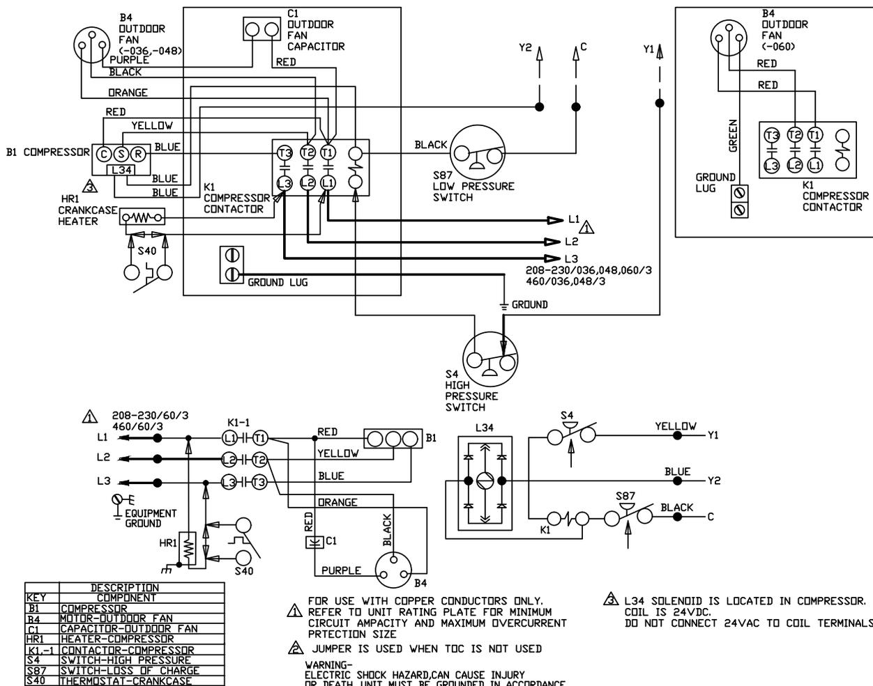
FIGURE 14. Typical Field Wiring Diagram -036, -048 (Y and G Voltage), -060 (Y Voltage)
