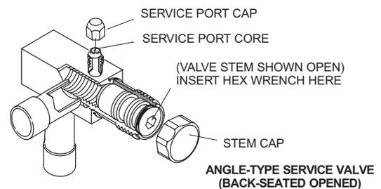
When service valve is **OPEN**, the service port is open to line set, indoor and outdoor unit.
