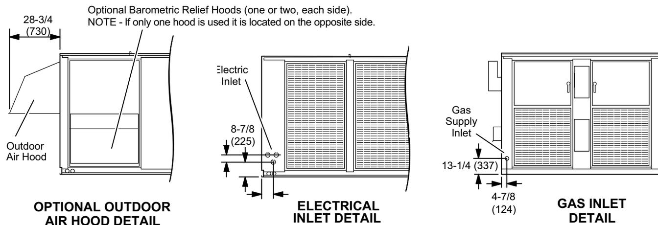
**LGH/LCH420, 480, 540, 600 Unit Dimensions Horizontal Airflow - In. (mm) - Gas Heat Shown**
