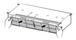
2. Clean the Air filter with a vacuum cleaner or soft brush. If dust is too heavy, then rinse it with running water and dry it in a ventilated area.
