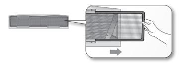
2. Clean the Air filter with a vacuum cleaner or soft brush. If dust is too heavy, then rinse it with running water and dry it in a ventilated area.
