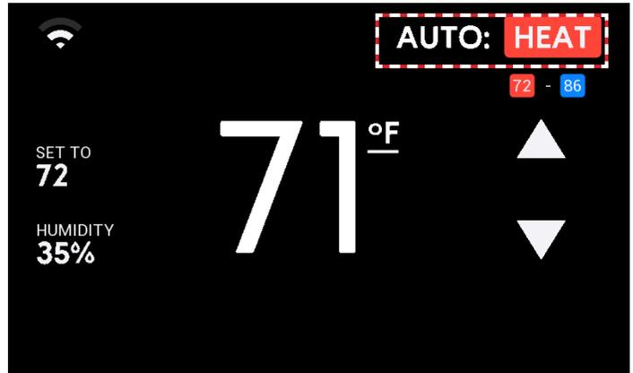
**Figure 28. Touch the Mode of Operation**
