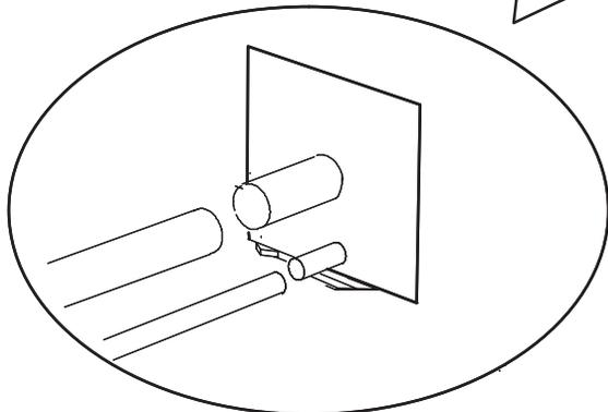
**F** PLACEZ UN CHIFFON HUMIDE CONTRE LA PLAQUE DES CONDUITES ET AUTOUR DE LA CONNEXION DE LA CONDUITE D'ASPIRATION.
