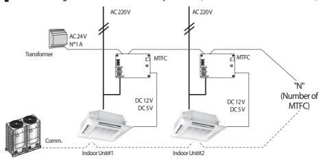
▶ When one transformer is installed with multiple MTFCs, current capacity setting should be 1 A x number of MTFC.
