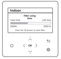
After cleaning and reinstalling the air filter, be sure to reset the filter-cleaning reminder as follows :
