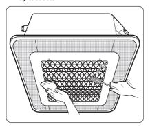
Wipe the surface of the unit with a slightly wet or dry cloth when needed. Wipe off dirt of odd-shaped areas by using a soft brush.
