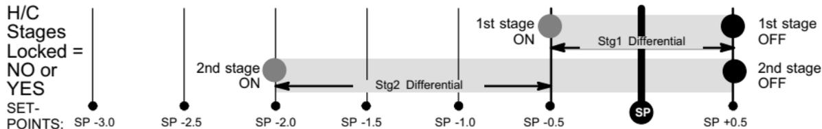
**Figure 18. Heating - dual fuel - 2 stage (1 compressor / 1 backup)**
