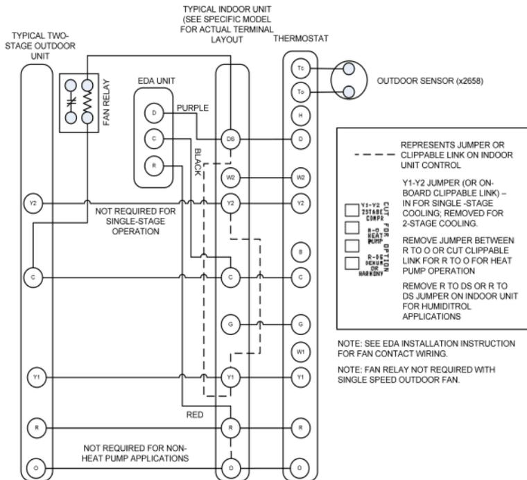
**Figure 3. Enhanced Dehumidification Accessory Typical Wiring Diagram**
