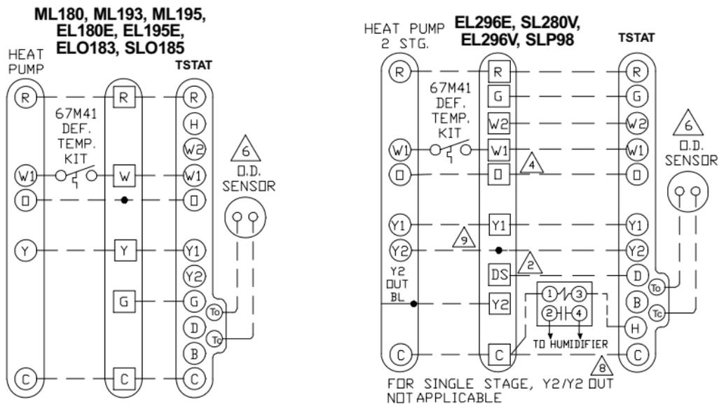
**Figure 11. Thermostat Wiring Diagrams (continued)**
