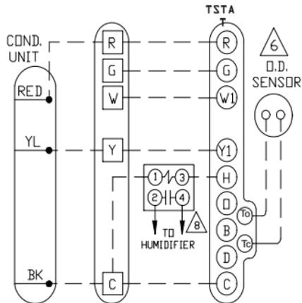
**Figure 7. Thermostat Wiring Diagrams (continued)**
