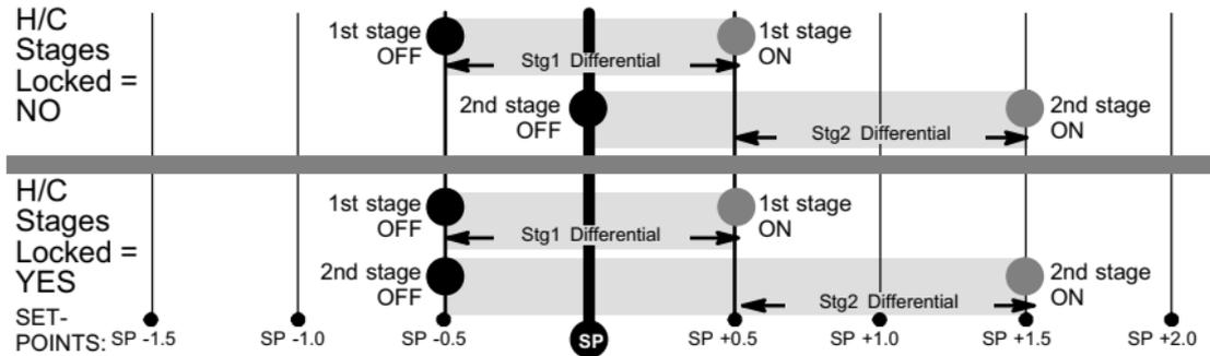
**Figure 14. Cooling - 1 or 2 stages**
