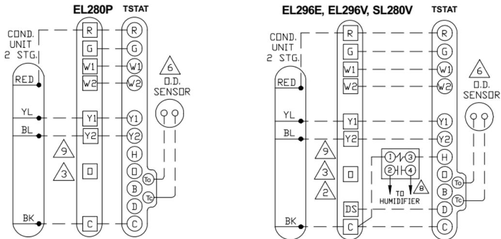
**Figure 9. Thermostat Wiring Diagrams (continued)**
