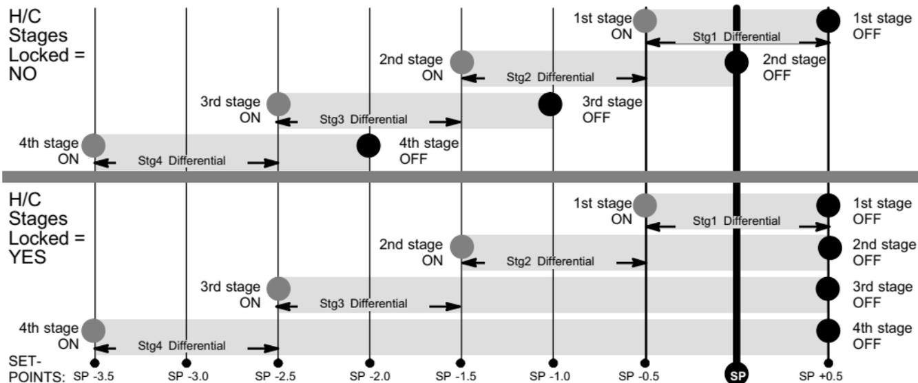
**Figure 17. Heating - Heat Pump w/electric - 4 stage (2 compressor / 2 backup)**
