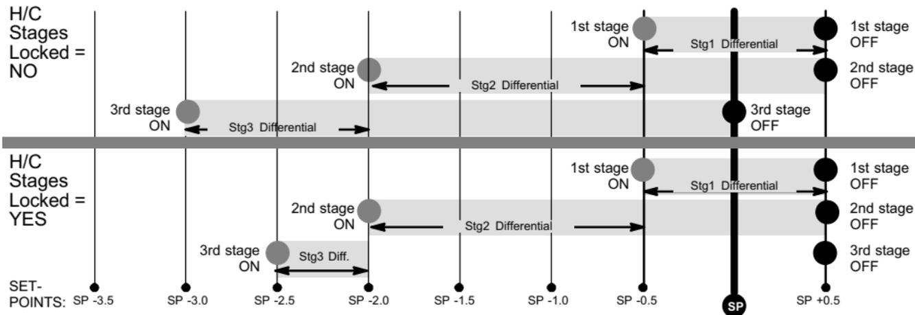
**Figure 19. Heating - dual fuel - 3 stage (1 compressor / 2 backup)**
