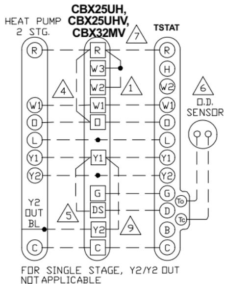
**Figure 10. Thermostat Wiring Diagrams (continued)**
