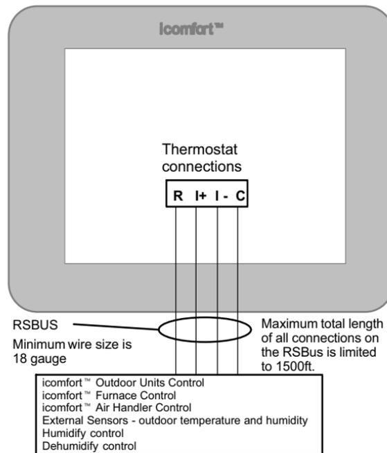
Figure 1. icomfort thermostat system
