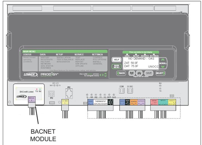
Figure 2. M3 Unit Controller BACnet Module (BP1)
