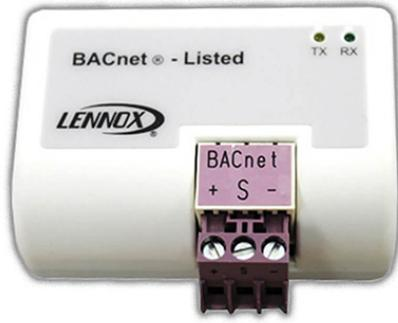
BACnet® Module (BP1) allows communication between the Lennox M2 and M3 Unit Controller and a BACnet® MS/TP network. This module is mounted directly to the M2 or M3 Unit Controller and is not compatible with M1-8 IMC and earlier versions.
