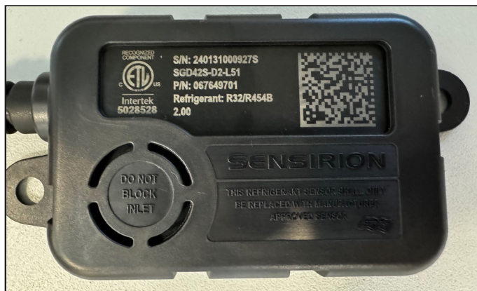
FIGURE 20. Example of Clear, Unobstructed Sensor Inlet
