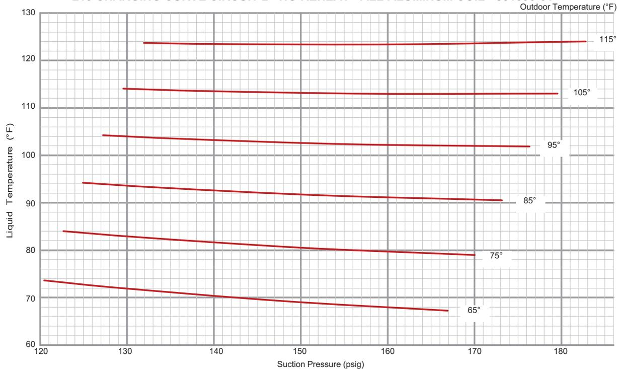
**210 CHARGING CURVE CIRCUIT 3 - NO REHEAT - ALL-ALUMINUM COIL - 581090-01**
