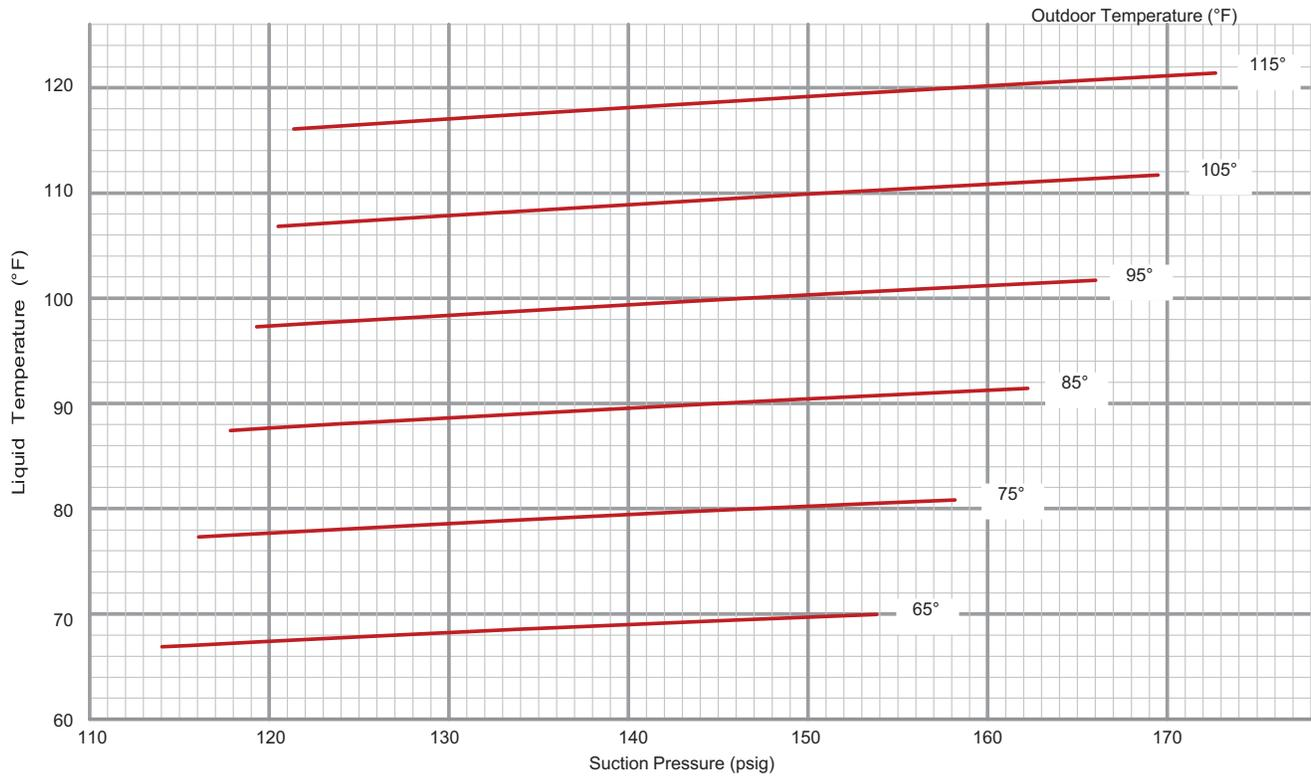
**240 CHARGING CURVE CIRCUIT 2 - NO REHEAT - ALL-ALUMINUM COIL - 581094-01**
