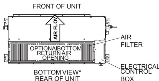
\*NOTE - Unit orientation reversed to show alternative filter location and return air path on bottom of unit.
