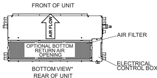
\*NOTE - Unit orientation reversed to show alternative filter location and return air path on bottom of unit.
