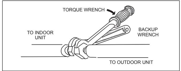
**Figure 36. Tighten Flare Nut**
