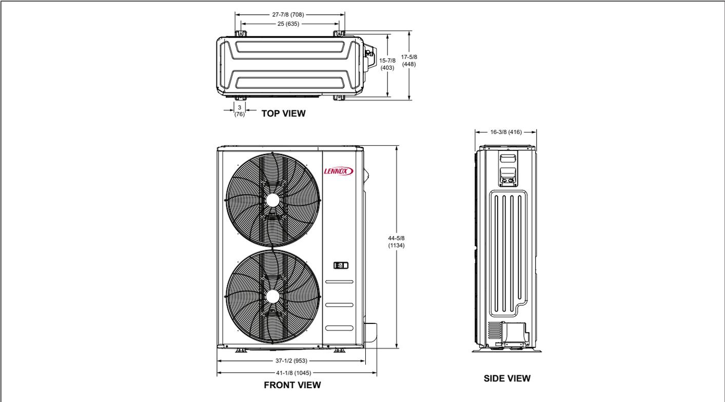
Figure 6. MPC048S4S Outdoor Unit Dimensions - Inches (mm)
