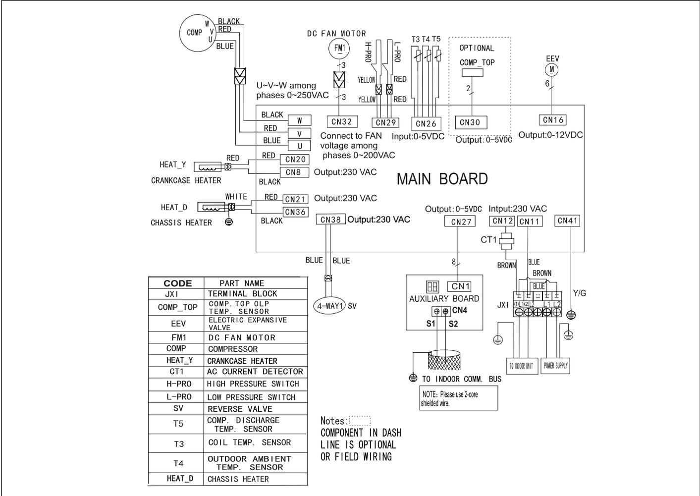
**Figure 42. 208/230V MPC036S4S-\*P Outdoor Unit Wiring Diagram**
