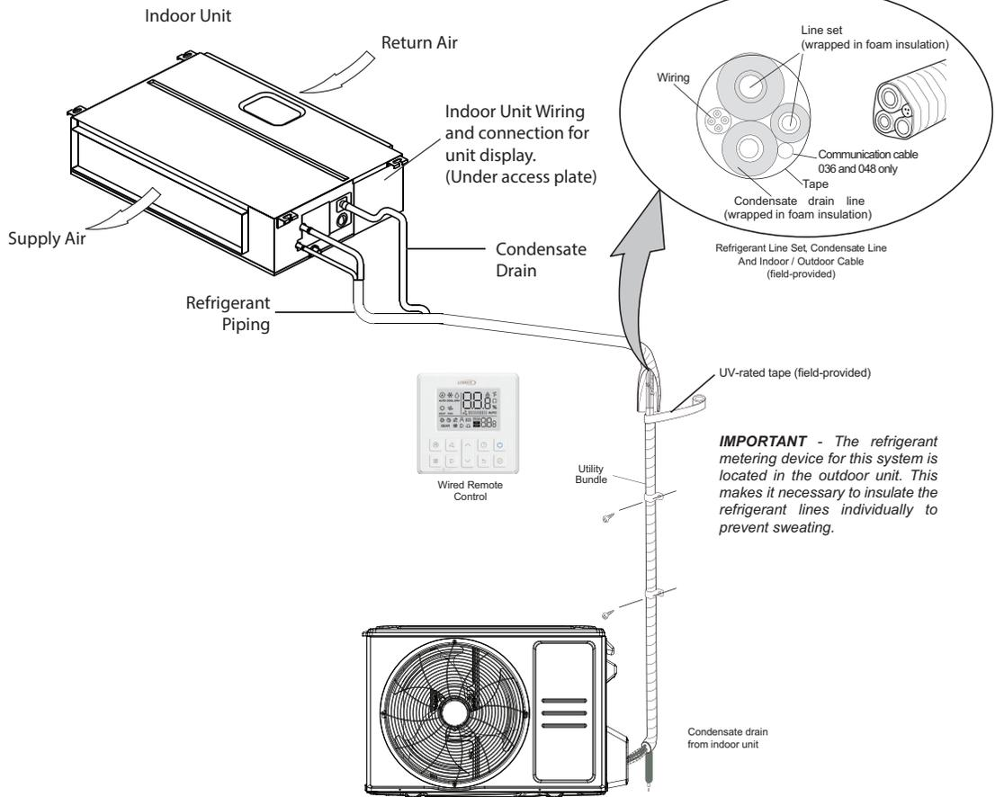
**IMPORTANT** - The refrigerant metering device for this system is located in the outdoor unit. This makes it necessary to insulate the refrigerant lines individually to prevent sweating.
