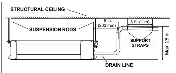
Figure 20. Condensate Drain with Factory Condensate Pump
