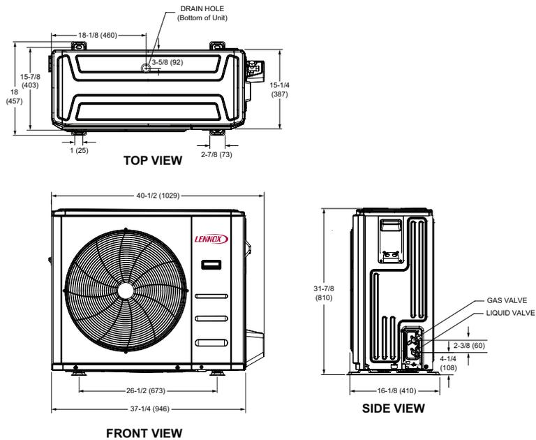
**Figure 9. MLB024S4S Outdoor Unit Dimensions - Inches (mm)**
