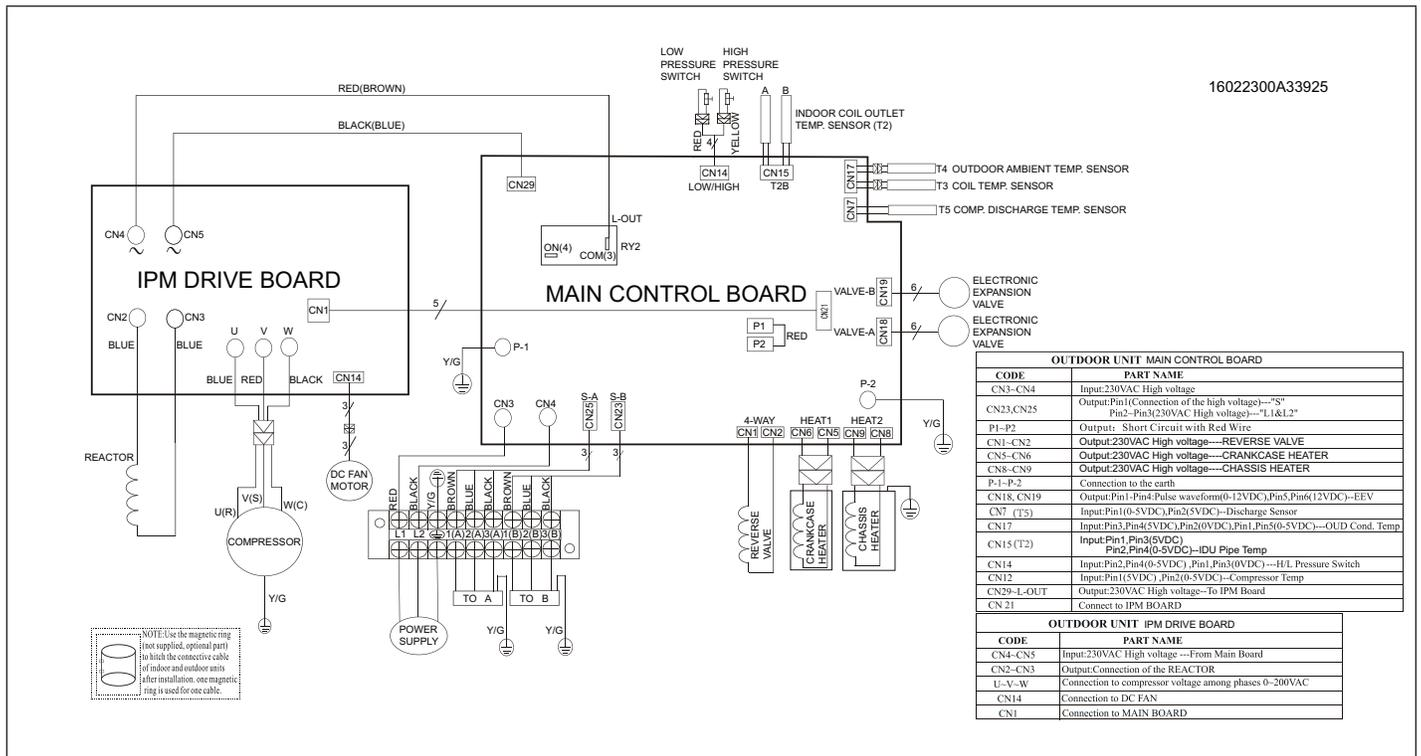
Figure 45. 208/230V MLB018S4S-\*P Outdoor Unit Wiring Diagram
