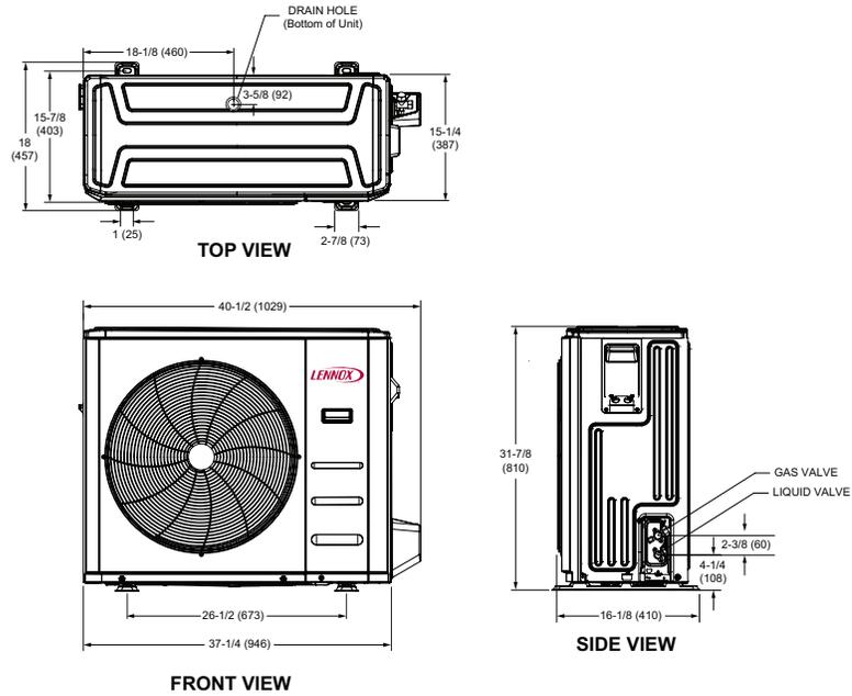
Figure 5. MPC036S4S Outdoor Unit Dimensions - Inches (mm)
