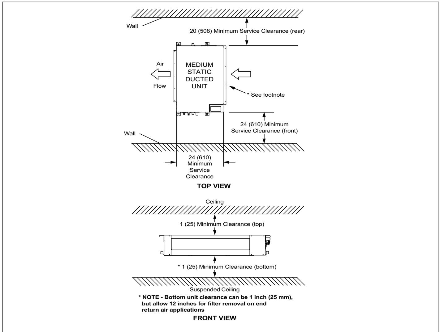
Figure 13. Indoor Unit Clearances - Inches (mm)
