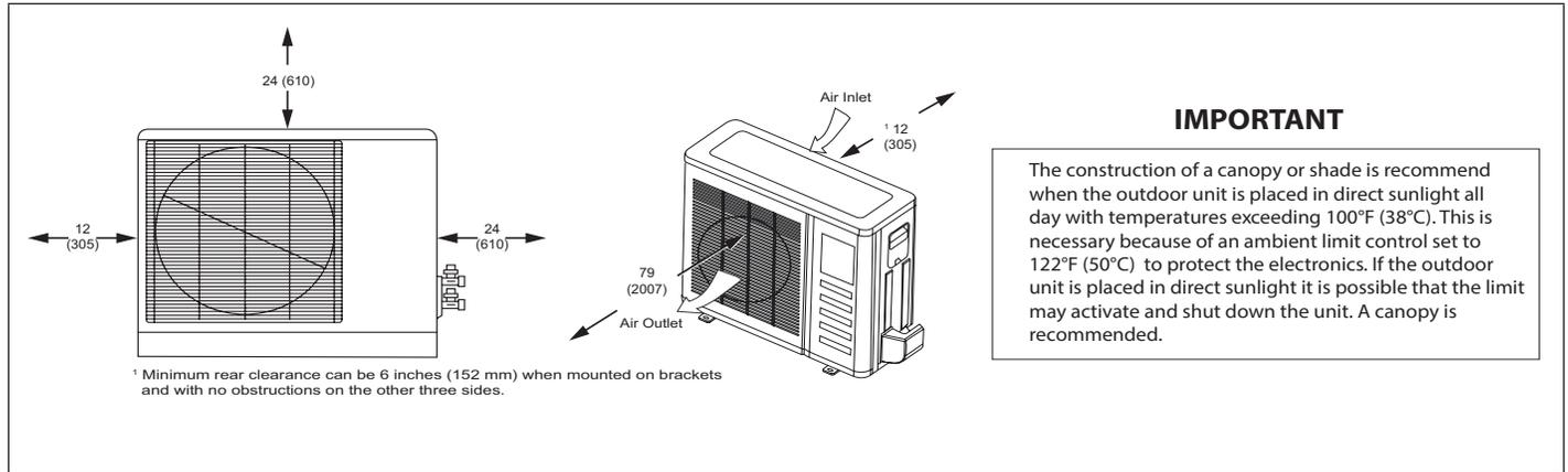
Figure 12. Outdoor Unit Clearances - Inches (mm)
