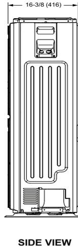
**Figure 10. Outdoor Unit Dimensions (MLB036S4S-\*P, MLB048S4S-\*P) - Inches (mm)**
