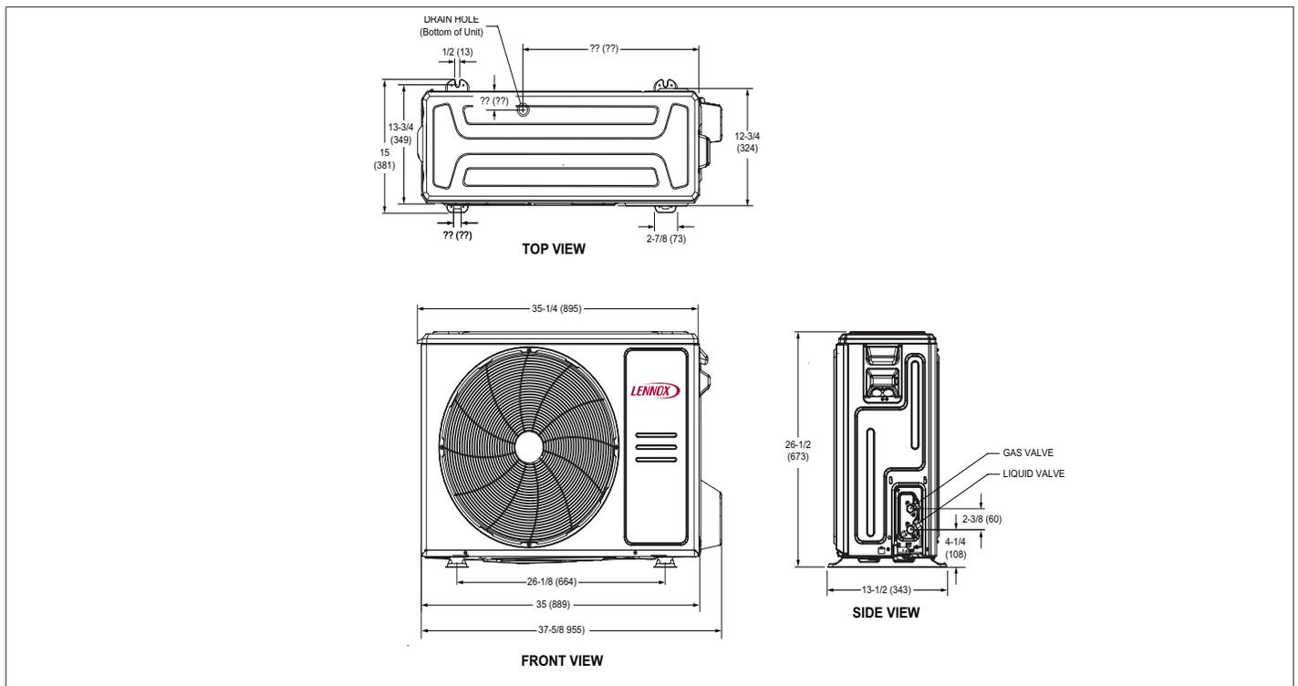
Figure 3. MPC018S4S Outdoor Unit Dimensions - Inches (mm)
