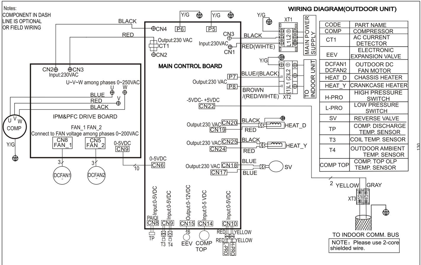
Figure 43. 208/230V MPC048S4S-\*P Outdoor Unit Wiring Diagram
