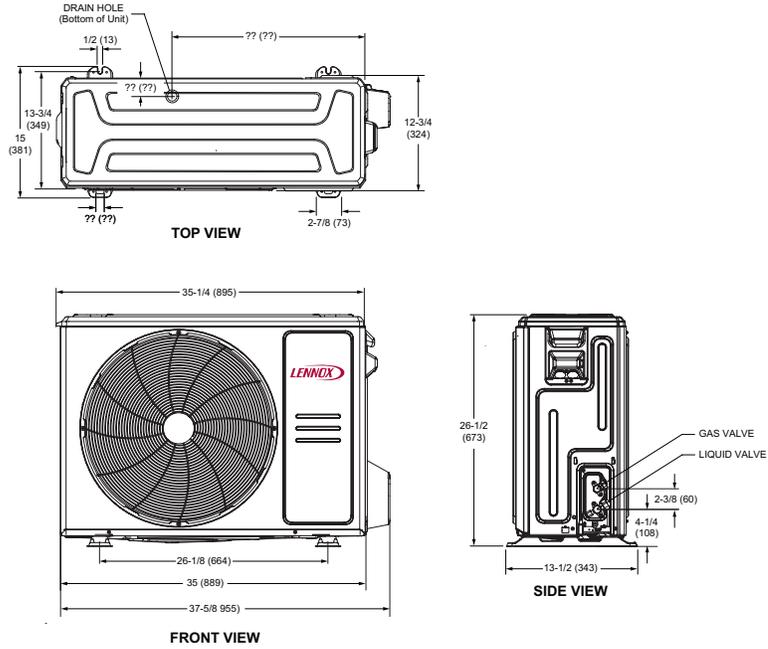
**Figure 8. MLB018S4S Outdoor Unit Dimensions - Inches (mm)**
