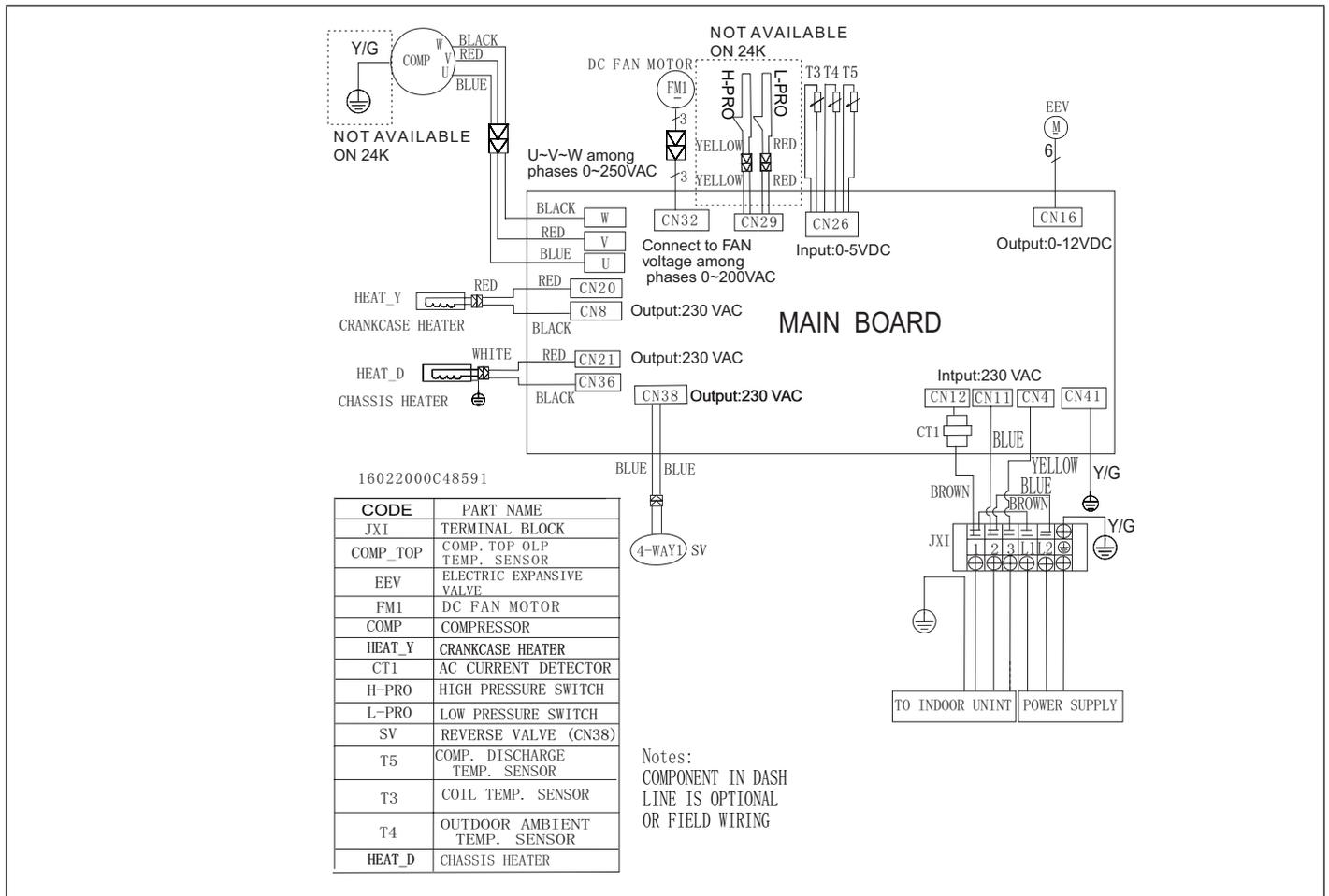
Figure 46. 208/230V MLB024S4S-\*P Outdoor Unit Wiring Diagram
