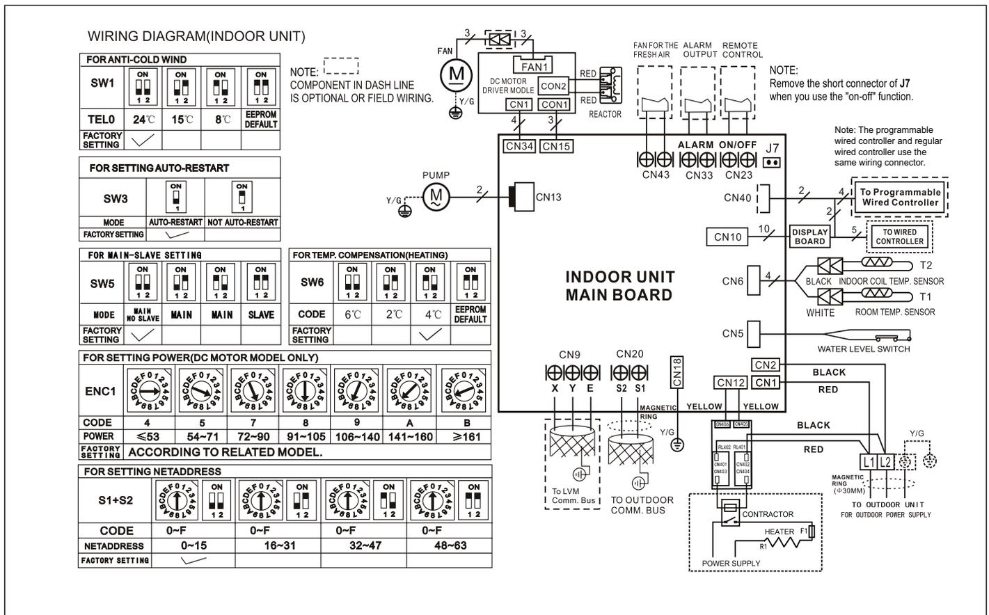
Figure 38. MMDB036S4-\*P and MMDB048S4-\*P Ducted Units Wiring Diagram
