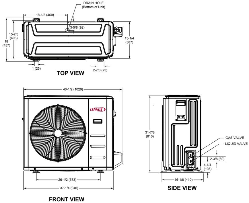
Figure 4. MPC024S4S Outdoor Unit Dimensions - Inches (mm)
