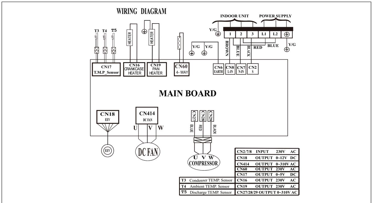
Figure 40. 208/230V MPC018S4S-\*P Outdoor Unit Wiring Diagram
