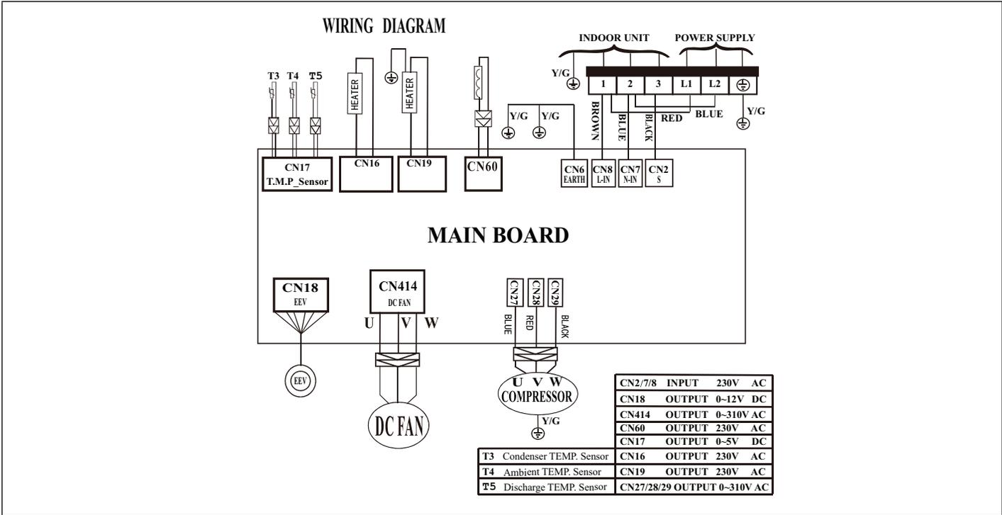
**Figure 41. 208/230V MPC024S4S-\*P Outdoor Unit Wiring Diagram**
