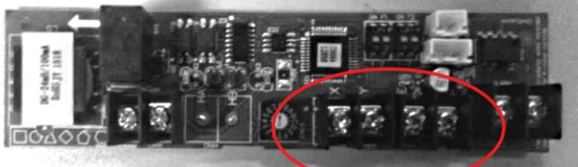
MPMC/MWCB/MWHB receiver board uses terminals for the programmable wired controller.
