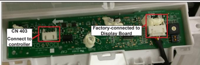
**NOTE** - CN 403 is used to connect either the M0STAT64Q local controller OR a centralized control. It is not possible to connect both the M0STAT64Q controller and a centralized control to this unit.
