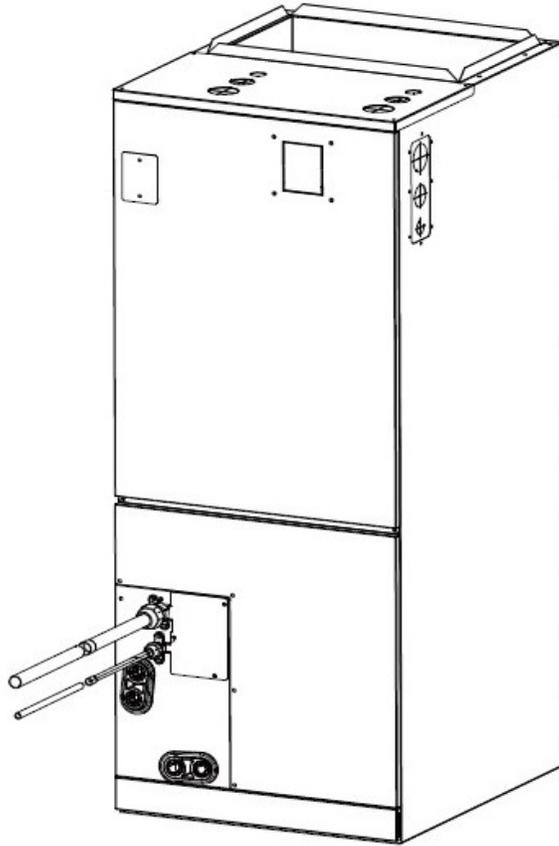
**Figure 6. Refrigerant Piping Connections**
