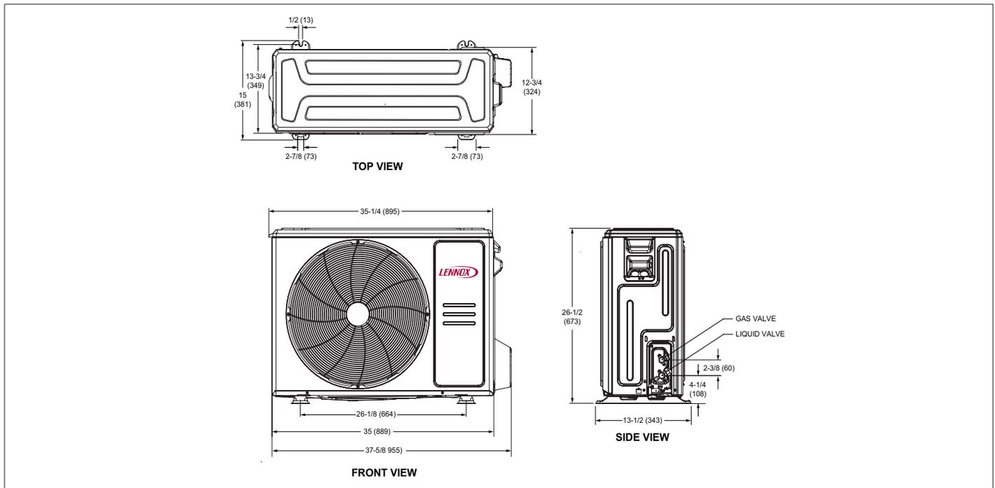
Figure 13. MLB018S4S Outdoor Unit Dimensions - Inches (mm)
