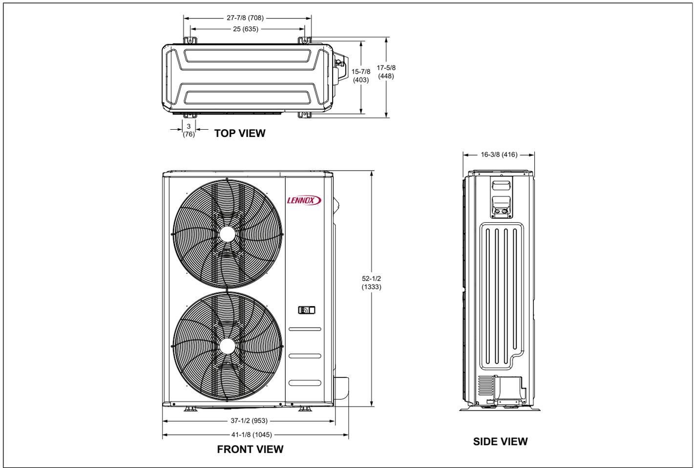
Figure 12. MPC048S4S and MPC060S4S Outdoor Unit Dimensions - Inches (mm)
