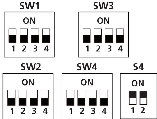
SW4 Dip Switch settings (Electric Heat Air Volume) adjusts the blower motor's nominal CFM based on the electric heat kit size. See "Electric Heat Air Volume Settings" on page 28.
