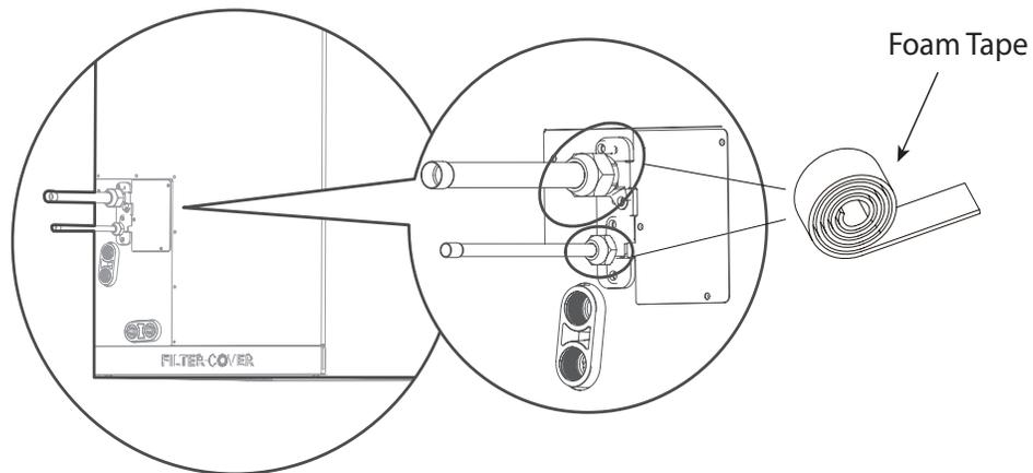
**Figure 7. Insulate Valve**
