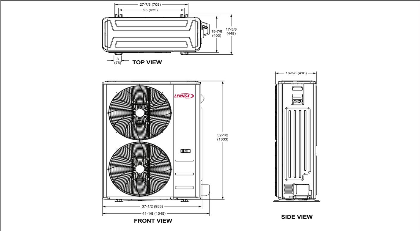
Figure 15. Outdoor Unit Dimensions (MLB036S4S-\*P and MLB048S4S-\*P) - Inches (mm)
