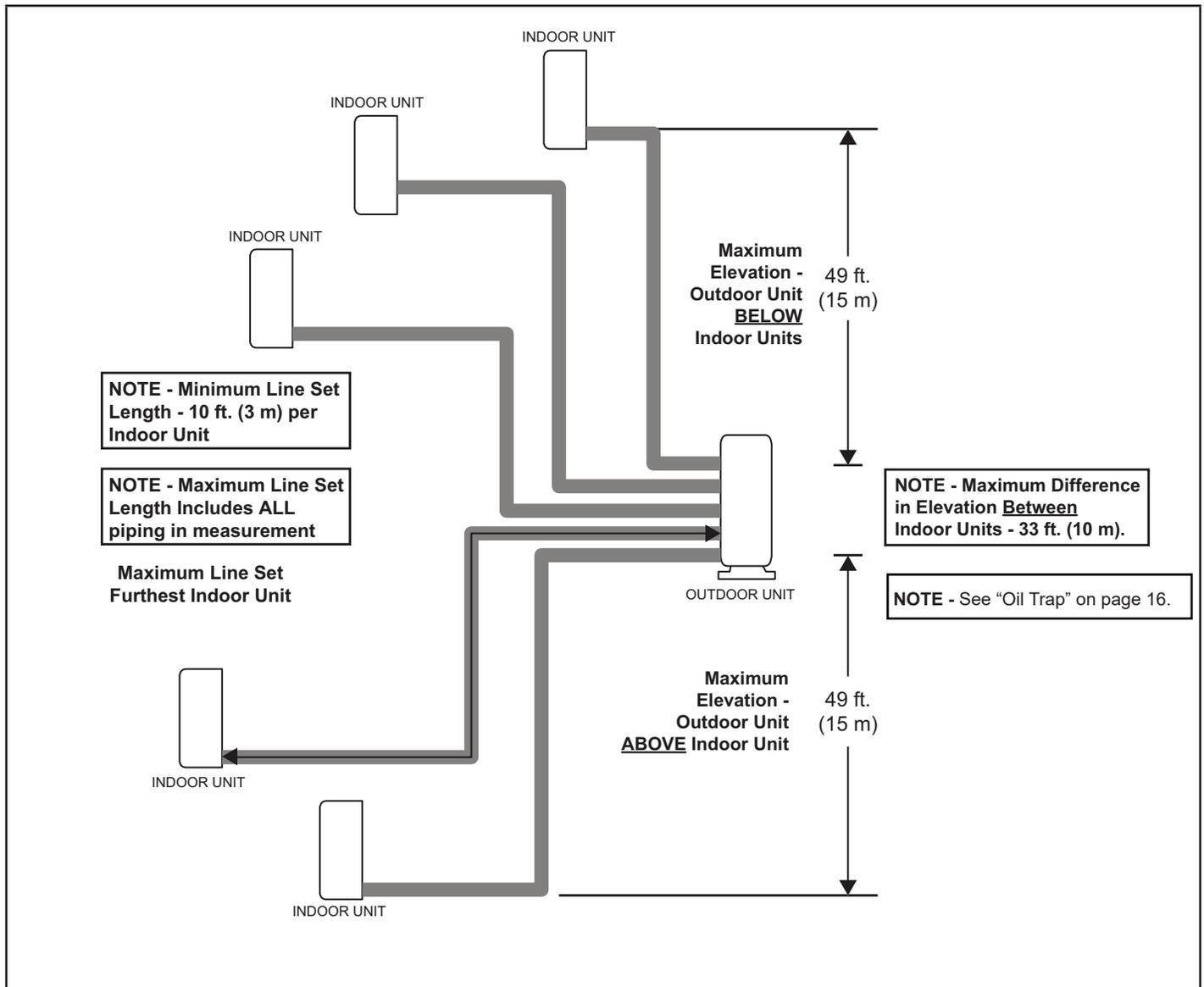
Figure 30. MPC and MLB Line Set Elevations
