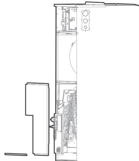
4. Unplug temperature sensors T1, T2 from the control board.
