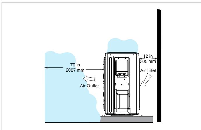
**Figure 20. Outdoor Unit Air Flow Obstructed by Snow (Typical)**
