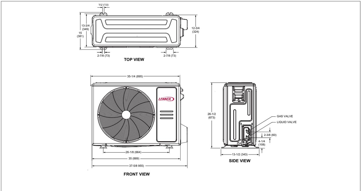
Figure 10. MPC018S4S Outdoor Unit Dimensions - Inches (mm)
