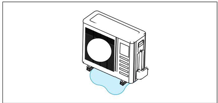
**Figure 21. Avoid Defrost Water Ice Hazard (Typical)**
