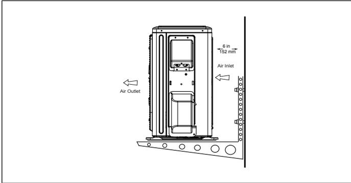
**Figure 28. Securing Outdoor Unit to Brackets (Typical)**
