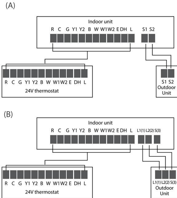
Figure 9. 24V Thermostat Diagram
