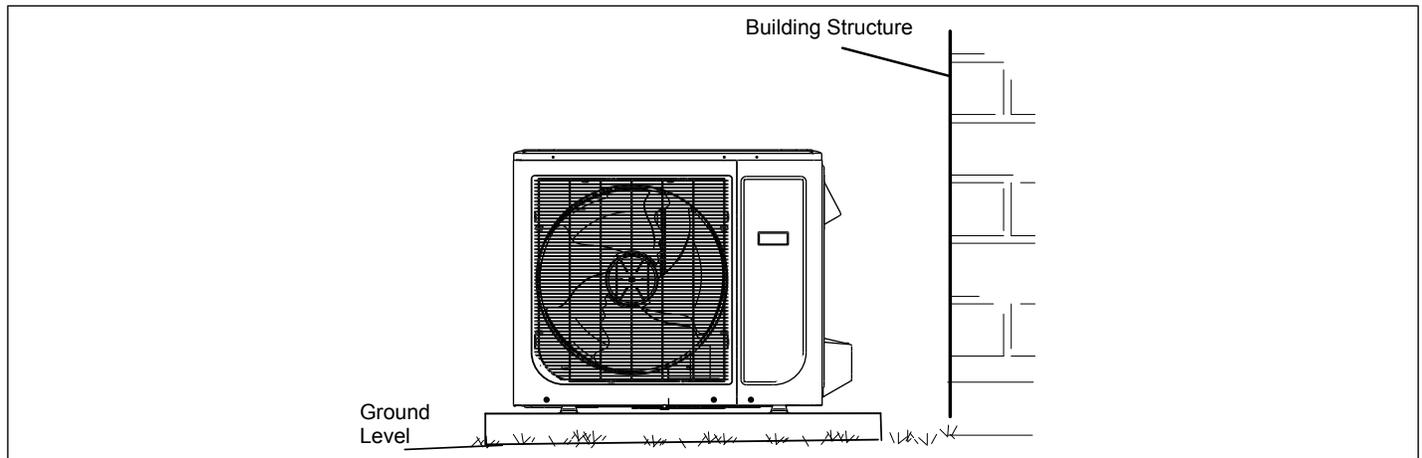
**Figure 17. Install Unit Level (Typical)**
