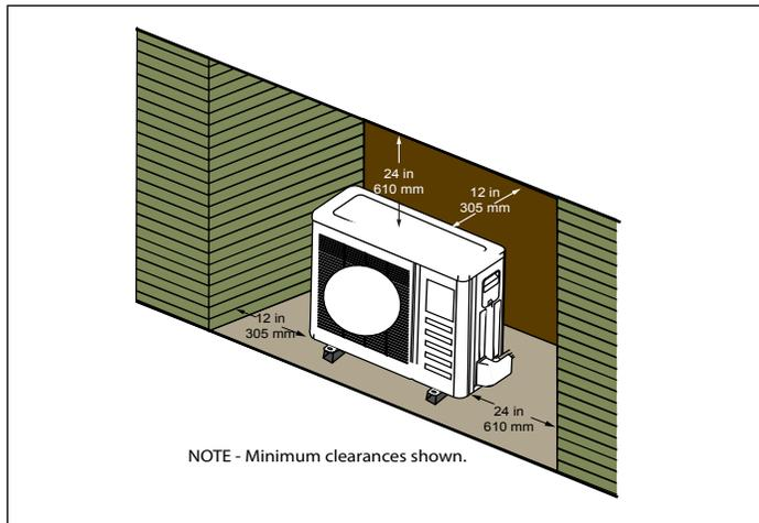
**Figure 24. Unit installed in Alcove (Typical)**
