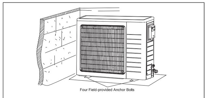
**Figure 26. Securing Outdoor Unit to Slab (Typical)**
