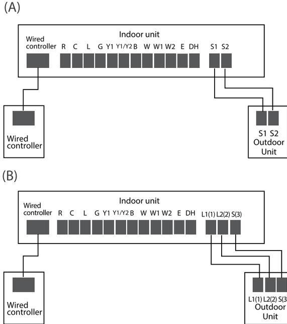
Figure 8. Wired Controller Diagram
