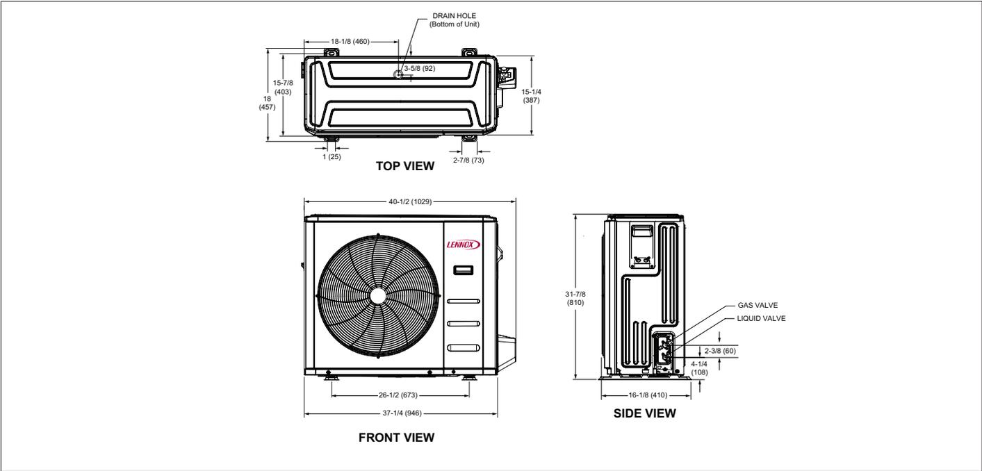
Figure 14. MLB024S4S Outdoor Unit Dimensions - Inches (mm)
