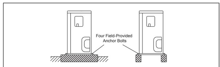
**Figure 27. Securing Outdoor Unit to Rails (Typical)**
