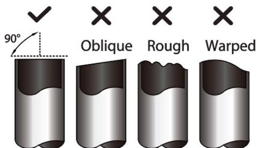
**NOTE:** Use extreme caution when cutting the pipe. Avoid damaging, denting, or warping the pipe while cutting it. Damaged pipes will drastically reduce the heating efficiency of the unit.
