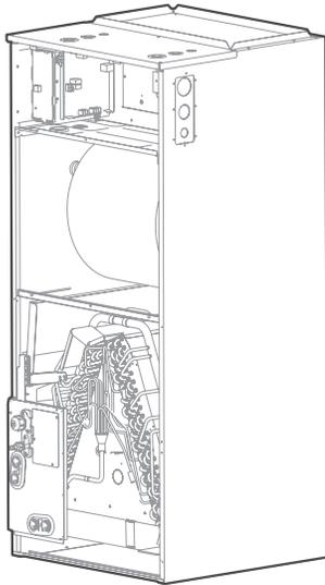
6. Remove the evaporator and drain pan; rotate it 180°.
