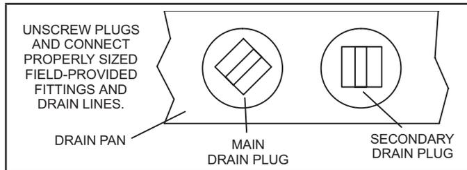
**Figure 4. Drain Line Connections**
