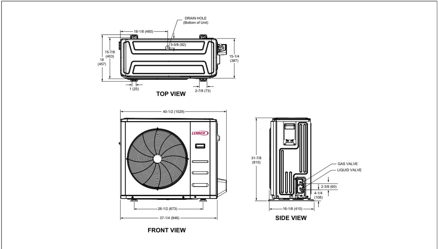
Figure 11. MPC024S4S, MPC030S4S, and MPC036S4S Outdoor Unit Dimensions - Inches (mm)
