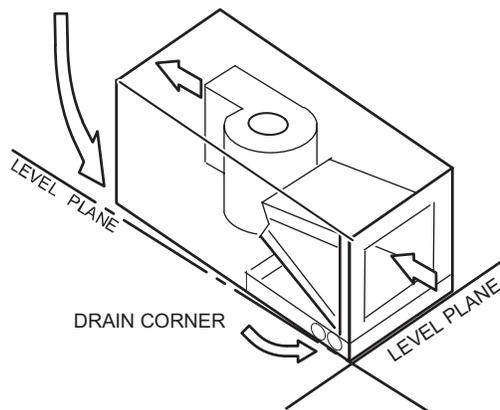
Figure 3. Sloping the Unit for Proper Drainage
