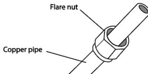
5. Remove PVC tape from ends of pipe when ready to perform flare work.
