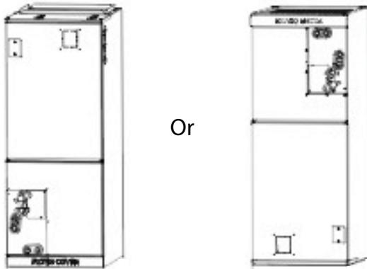
**NOTE:** When installed vertically (upward or downward), the lower end of the air outlet must be fastened by screws.
