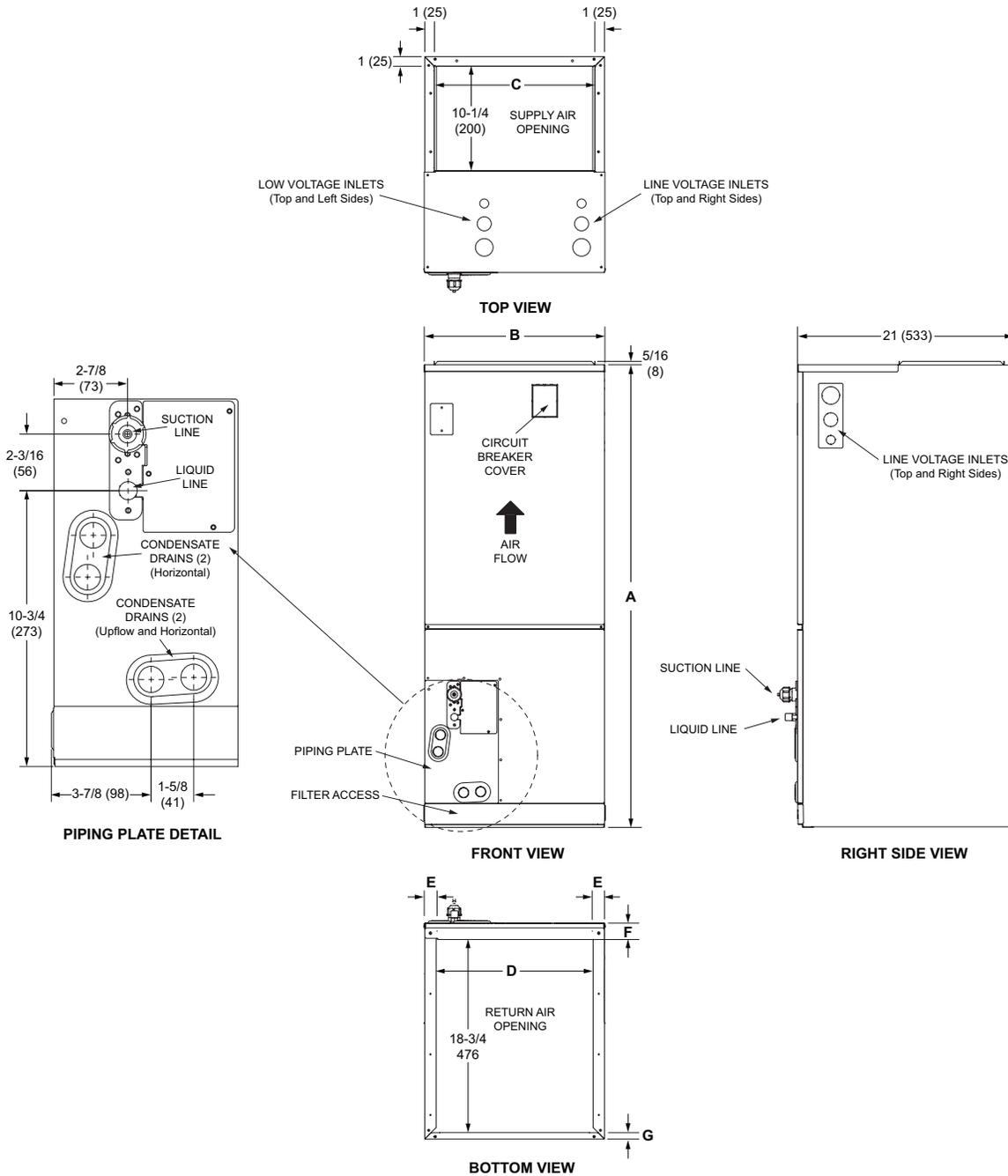
**NOTE:** Unit is shipped configured for horizontal left-hand air discharge. Unit may be converted to horizontal right-hand air discharge by repositioning horizontal drain pan. Dimensions remain the same in all configurations.
