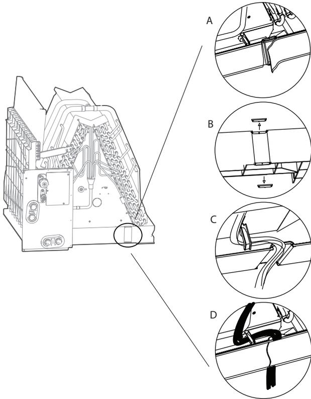
10. Use the cable ties to affix the Temperature Sensor back into place.
