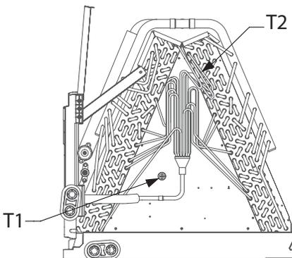
Figure 1. Temperature Sensor Locations
