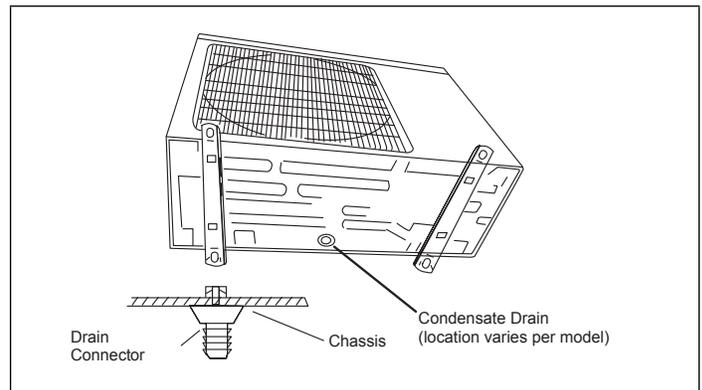
**Figure 25. Condensate Drain (Typical)**
