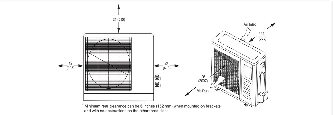
**Figure 16. Outdoor Unit Clearances - Inches (mm) - (Typical)**
