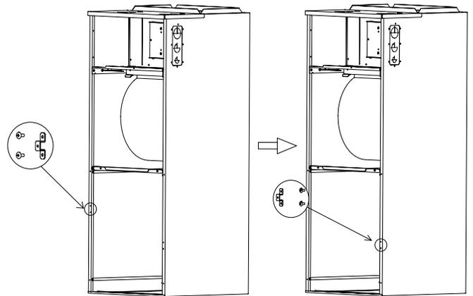
8. Reinstall the evaporator and drain pan.
