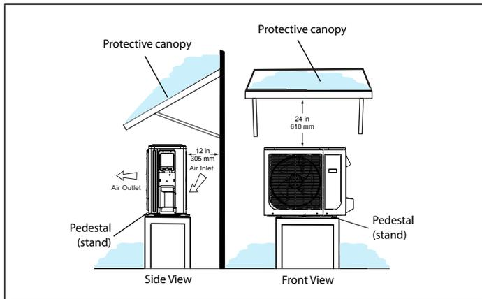
**Figure 18. Outdoor Unit on Pedestal (Stand) and Protective Canopy (Typical)**
