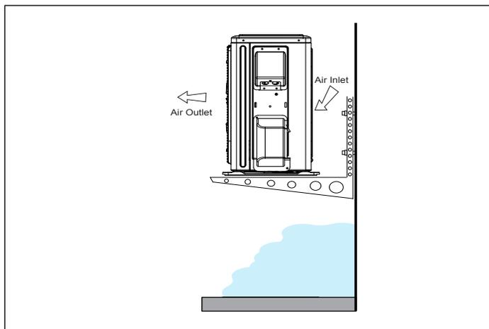
**Figure 19. Outdoor Unit on Brackets above Snow Line (Typical)**
