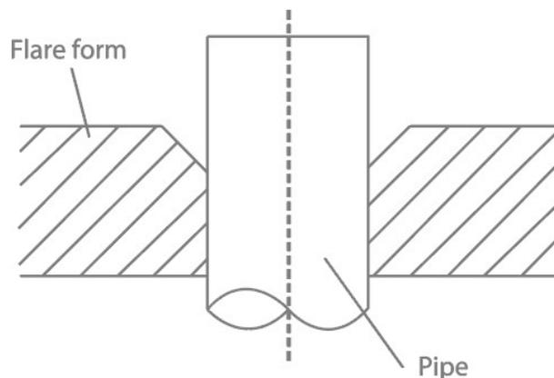
7. Place flaring tool onto the form.
