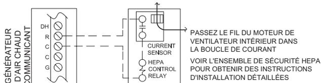
SYSTÈME DE CONTRÔLE DE LA VENTILATION LVCS
