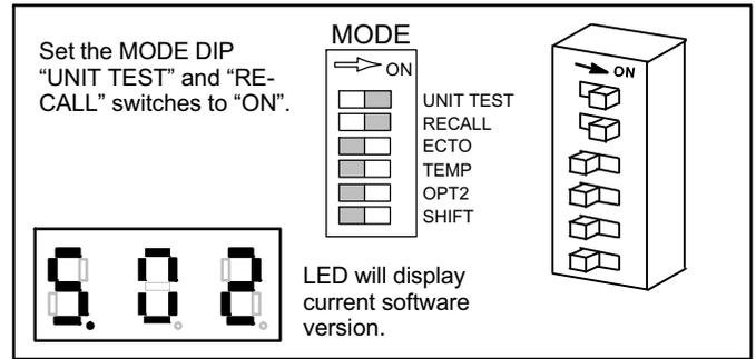
**Figure 4. Check Software Version and Address**
