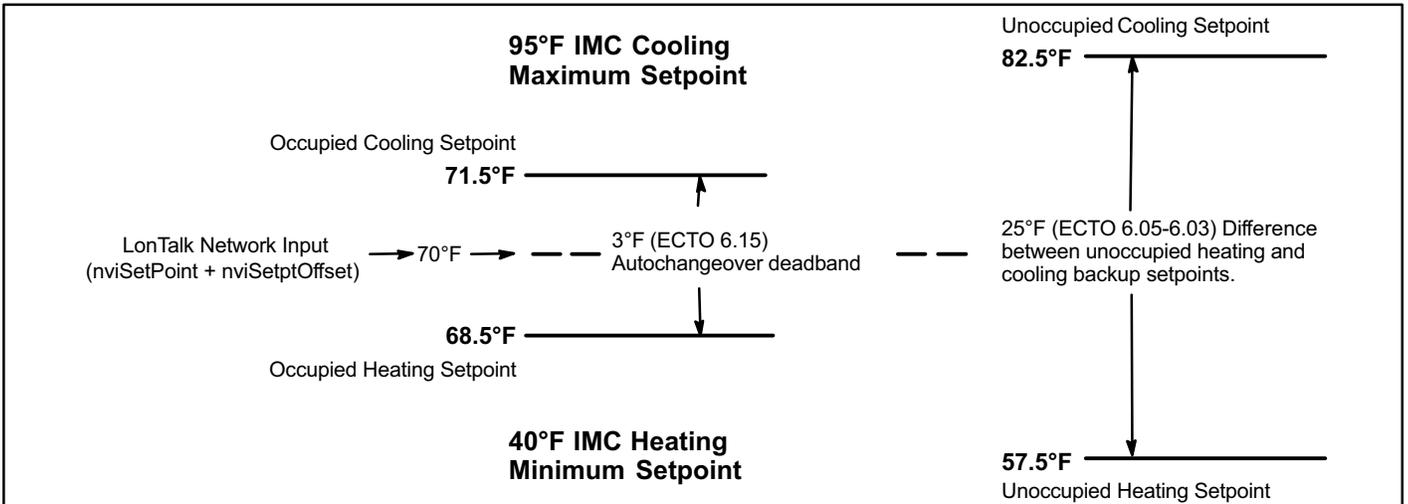
Figure 8. IMC Default Setpoint Example (Zone Sensor Installed)
