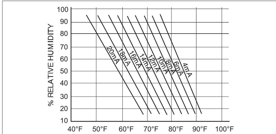
Figure 7. Enthalpy Sensor Output Current Honeywell C7400
