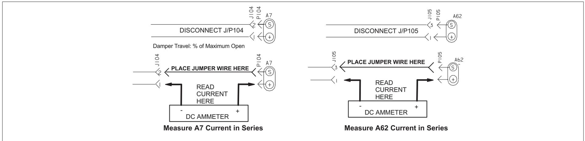
**Figure 8. Measure A7 and A62 Current in Series**
