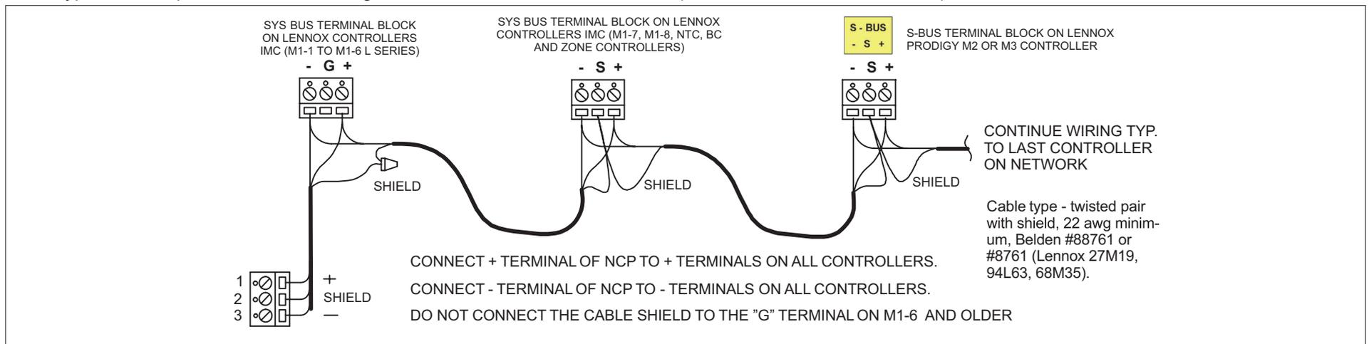
**Figure 12. L Connection® Network Daisy-Chain Communication Wiring**
