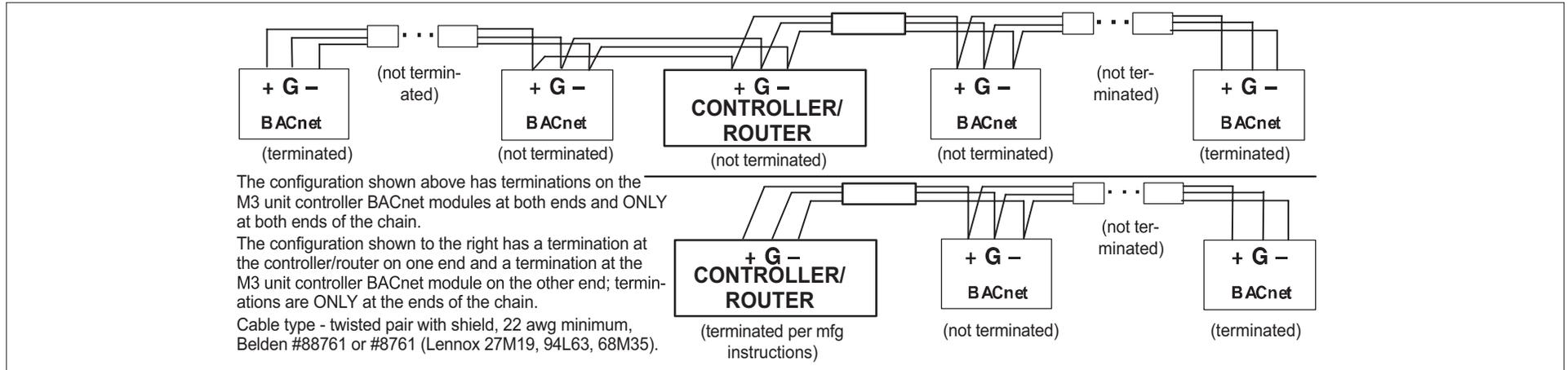
**Figure 11. Terminating Ends of a Daisy-Chain Network**
