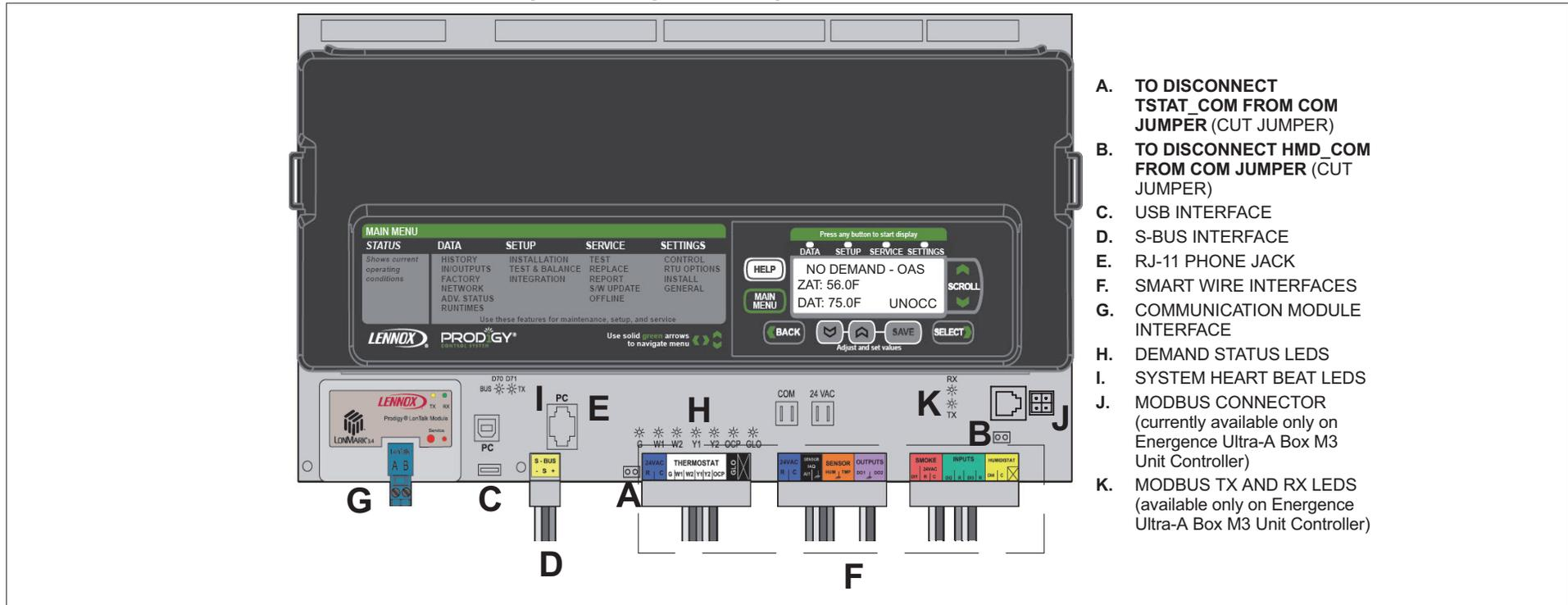
Figure 1. M3 Unit Controller Interfaces and LEDs Locations
