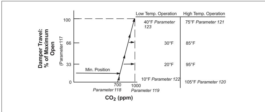
Figure 9. Default Demand Control Ventilation (DCV) Operation
