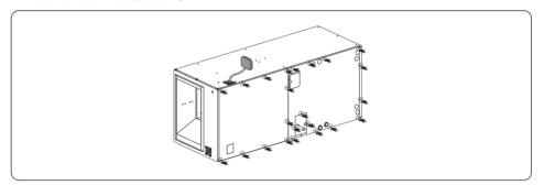
6 Fix the Wi-Fi module to the Ceiling to avoid the steel structure.
