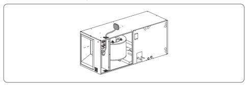
5 Assemble the front frame (23 screws)
