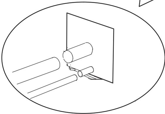
**F** PLACE A WET RAG AGAINST PIPING PLATE AND AROUND THE SUCTION LINE CONNECTION.
