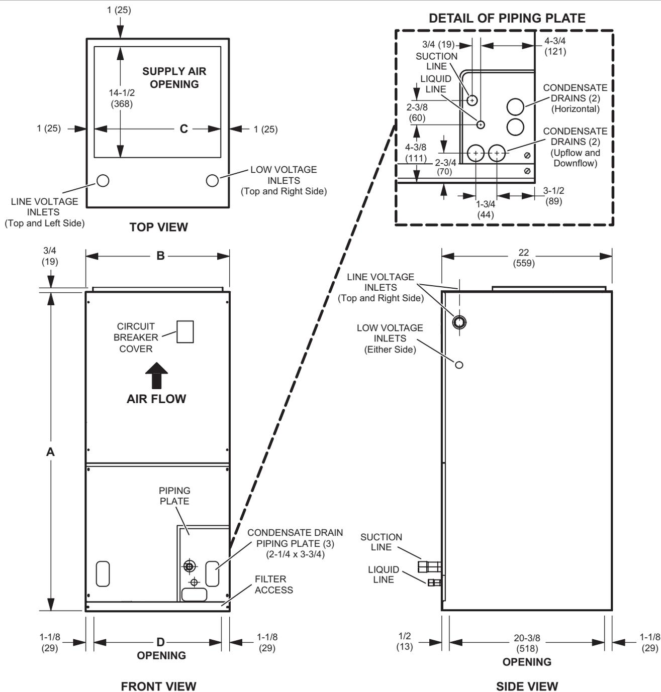
**NOTE** – Unit is shipped configured for horizontal right-hand air discharge. Unit may be converted to horizontal left-hand air discharge by repositioning horizontal drain pan. Dimensions remain the same in all configurations.
