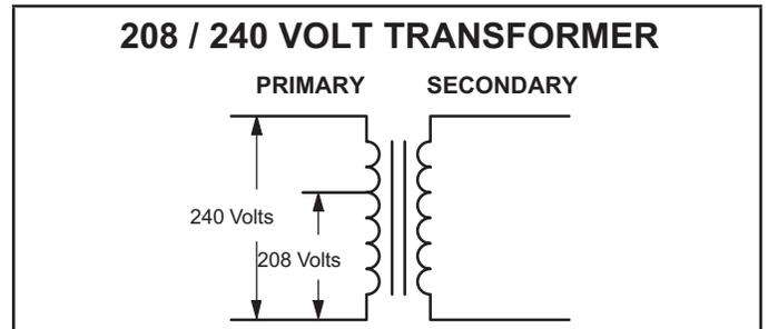
**FIGURE 13. Converting Unit from 240VAC to 208VAC**
