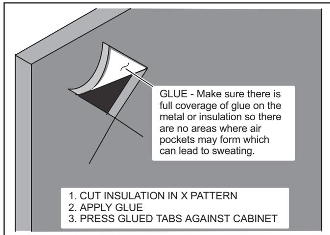
FIGURE 17. Repairing Insulation
