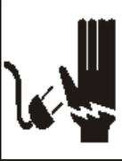
Electric shock hazard. Can cause injury or death. Before attempting to perform any service or maintenance, turn the electrical power to unit OFF at disconnect switch(es). Unit may have multiple power supplies.
