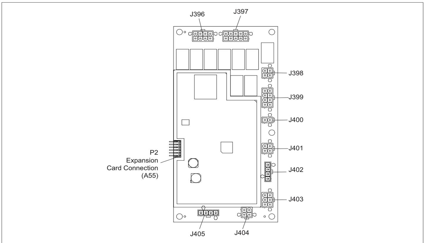
Figure 39. C4 Control Input and Outputs (A178)
