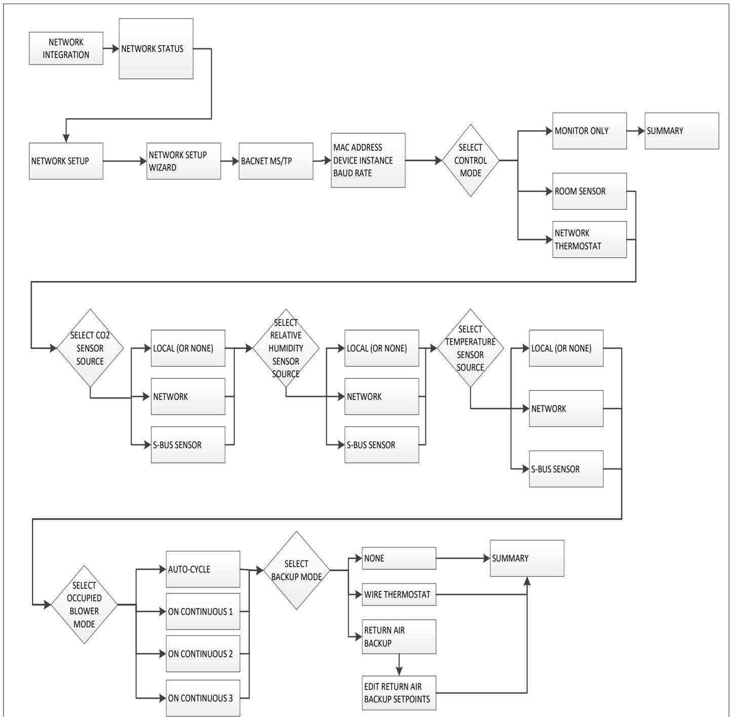
Figure 9. BACNet MS/TP Menu Structure
