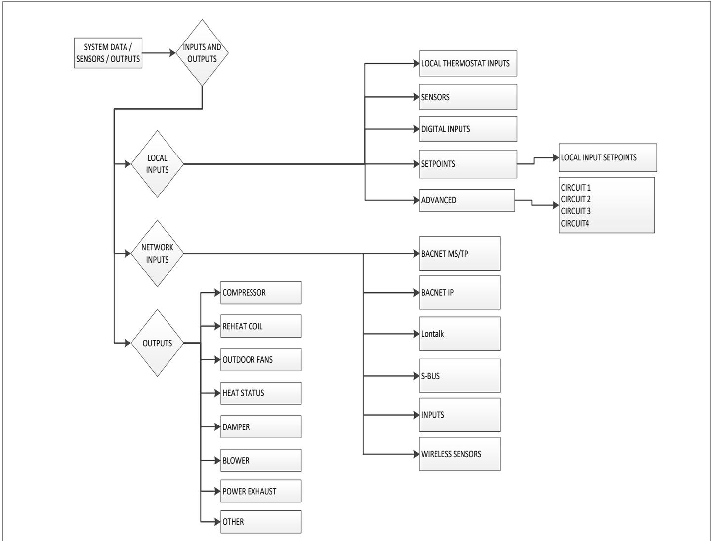
Figure 24. System Data / Sensors / Outputs Menu Structure
