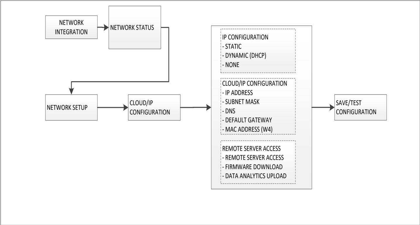
Figure 15. Cloud/IP Configuration Menu Structure
