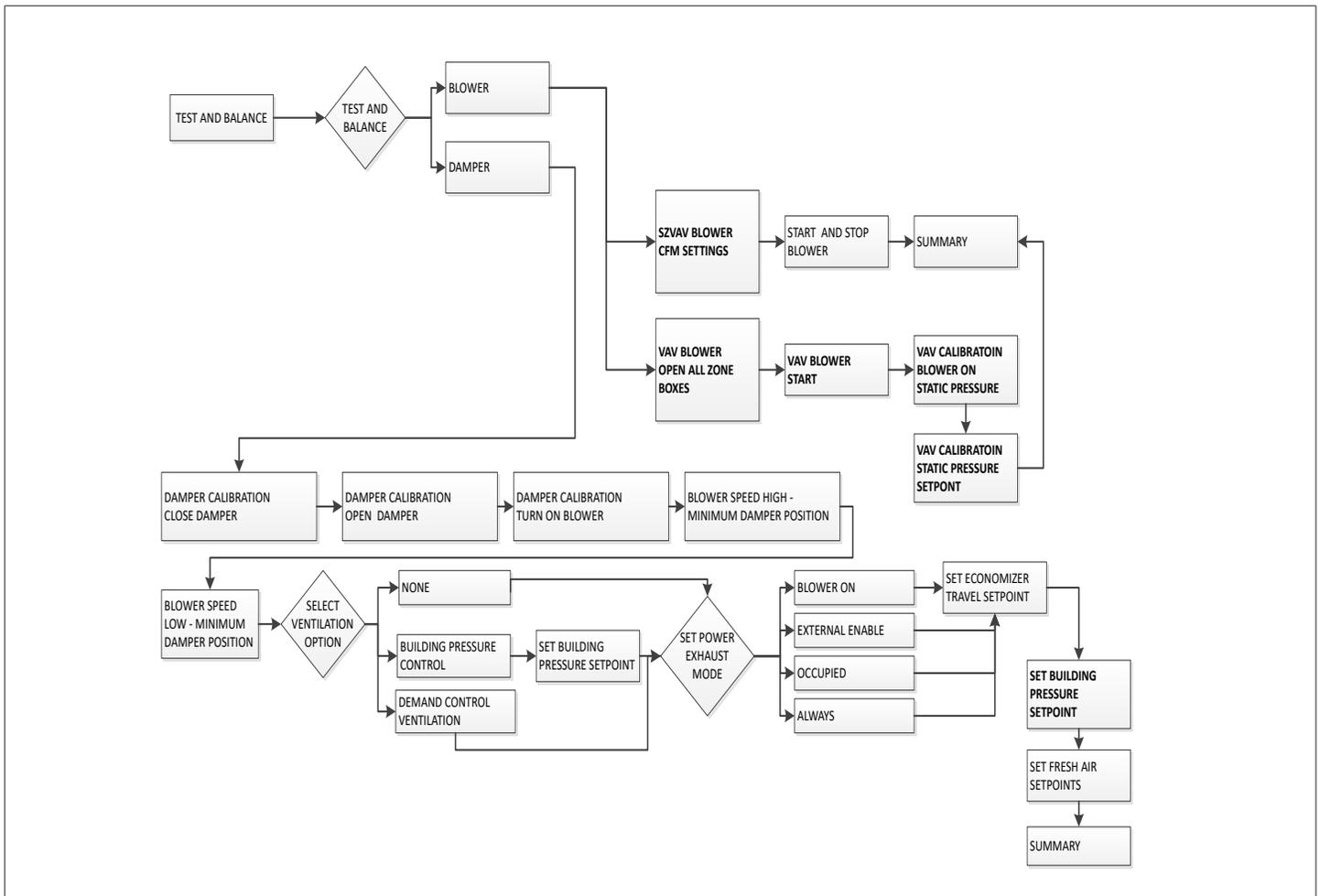
Figure 16. Motorized Outdoor Air Damper Only Menu Structure
