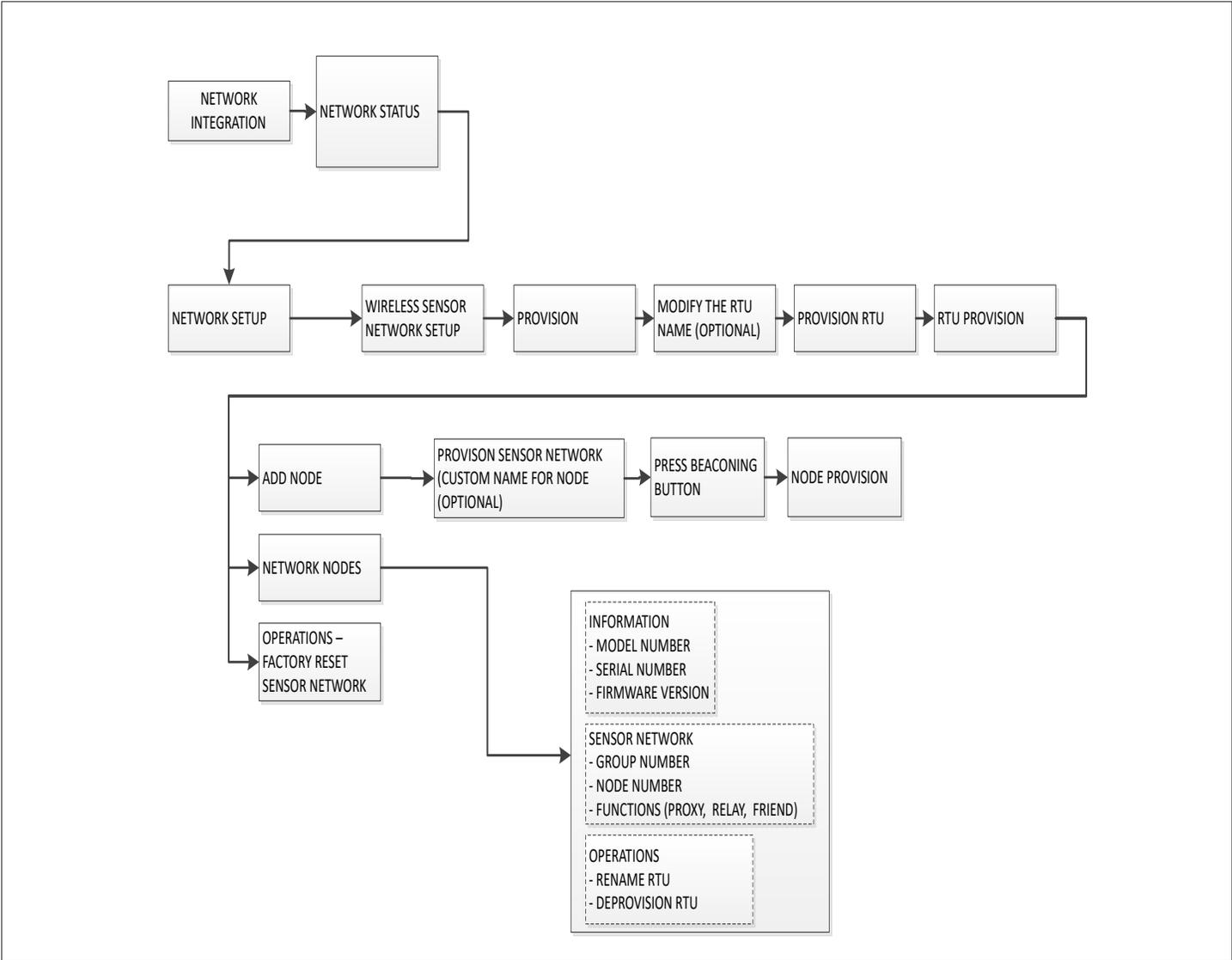
Figure 14. Wireless Sensor Network Setup Menu Structure
