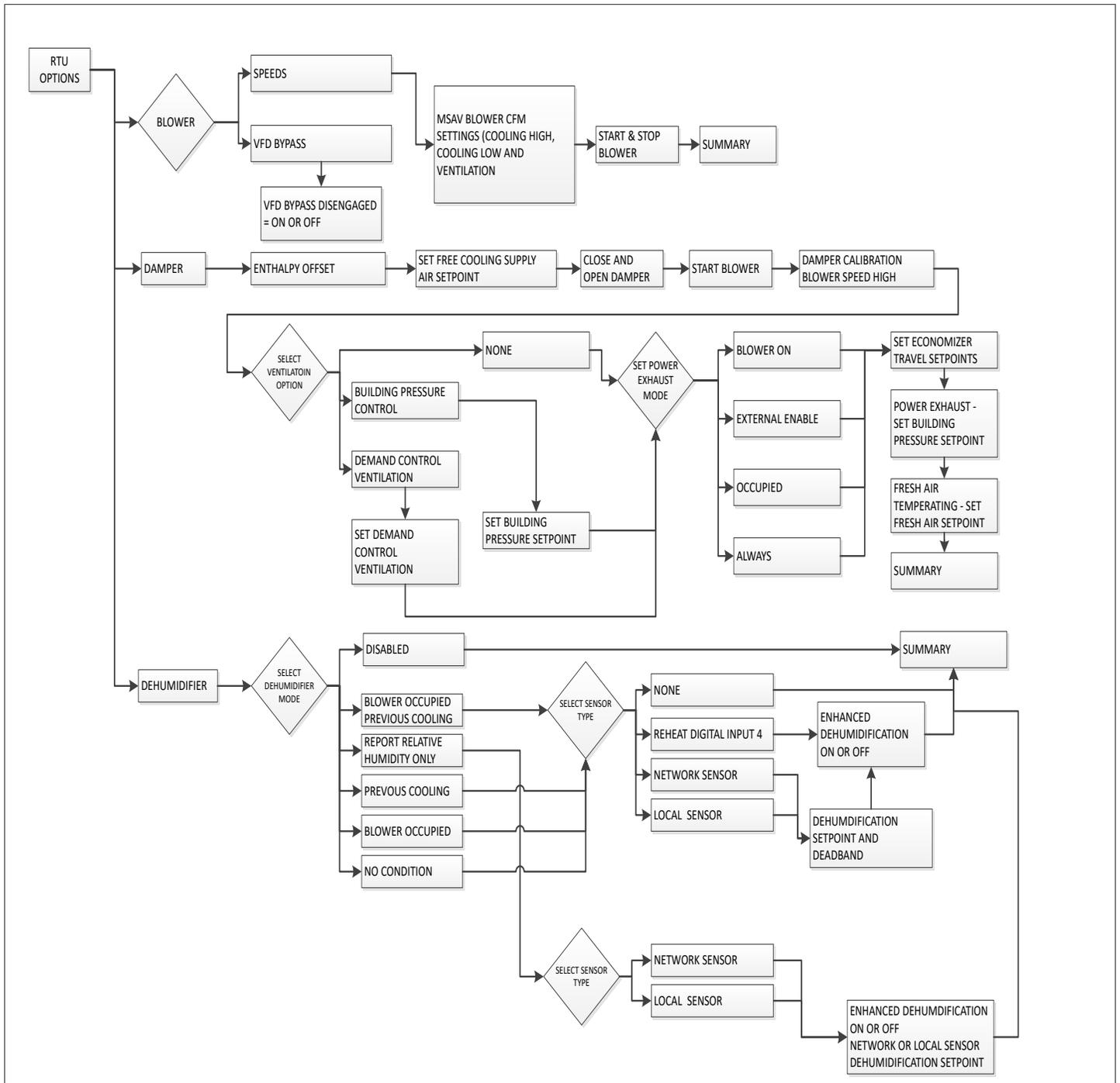
Figure 29. RTU Options - Blower, Damper and Dehumidifier
