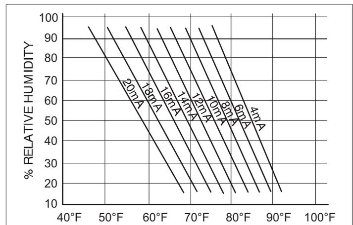
**Figure 32. Enthalpy Sensor Output Current Honeywell C7400**
