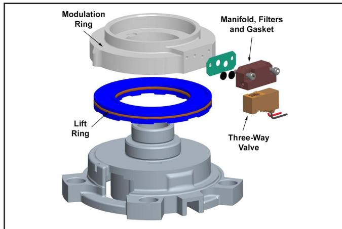
FIGURE 2. Two-Stage Scroll Compressor
