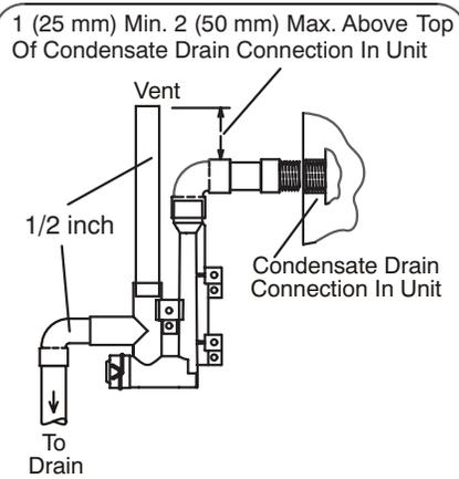
Drain Trap Assembly with 3/4 inch Piping
