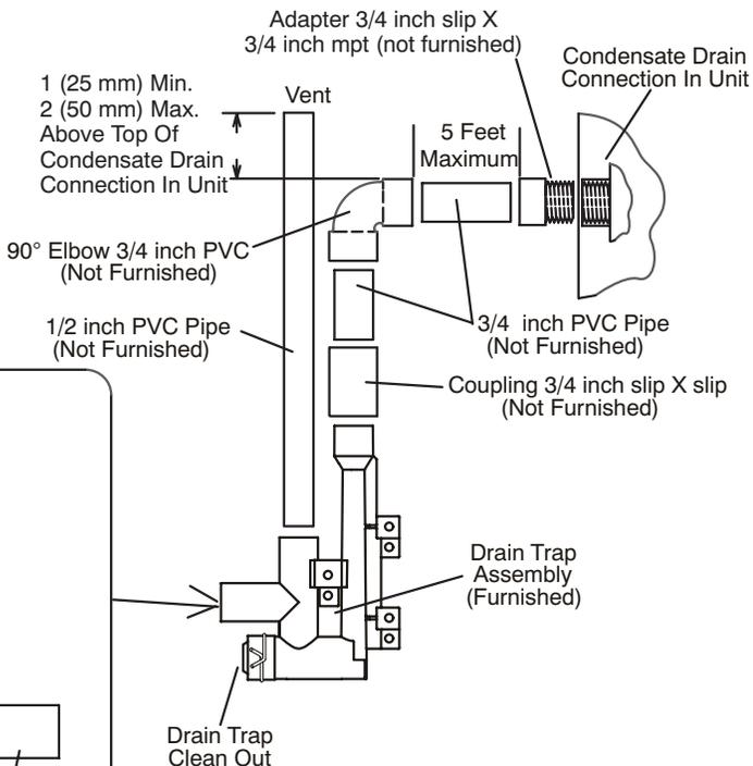
Drain Trap Assembly with 1/2 inch Piping
