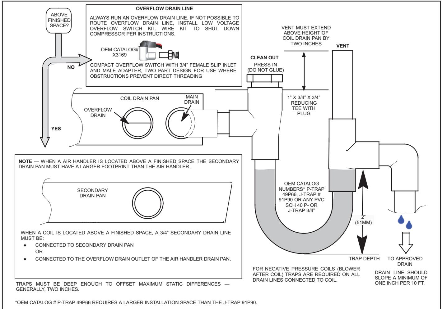
**FIGURE 6. Typical Main and Overflow Drain Installations**
