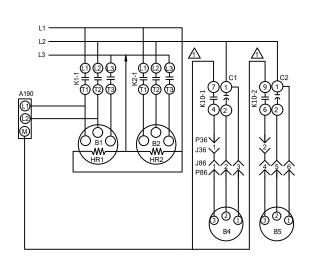
REMOVE EXISTING WIRES "K10-7" AND "K10-9" FROM RELAY CONNECTOR ON THE K10 RELAY. LOOSE WIRES MUST BE PROPERLY ISOLATED TO PREVENT AN ELECTRIC SHOCK HAZARD.
