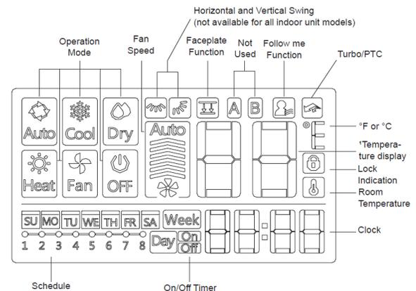
\* Displays cooling setpoint, heating setpoint or room temperature
