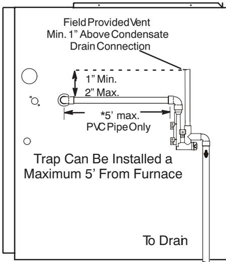
\*Piping from furnace must slope down a minimum 1/4" per ft. toward trap
