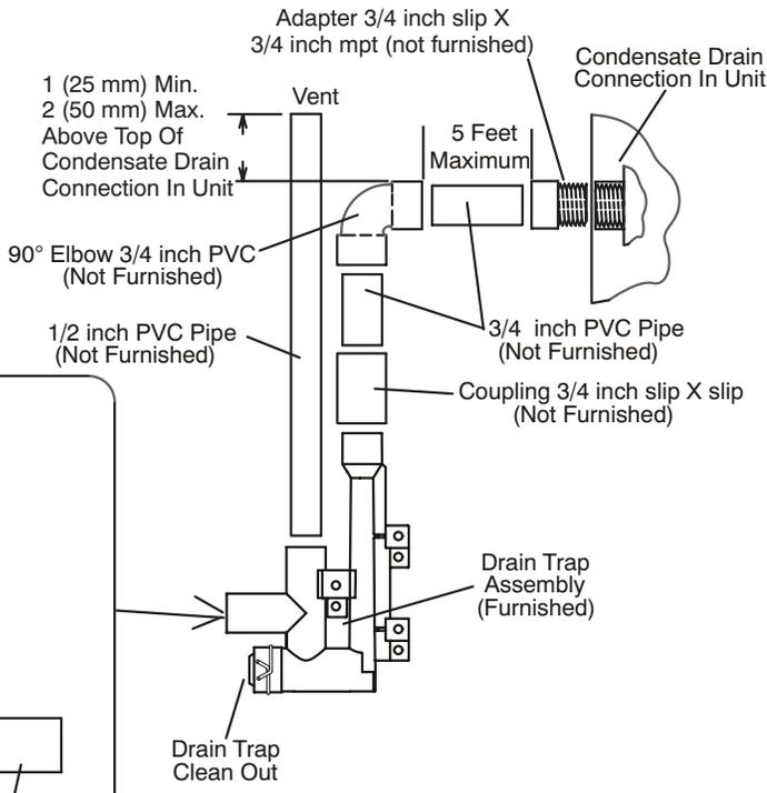
**Drain Trap Assembly with 1/2 inch Piping**
