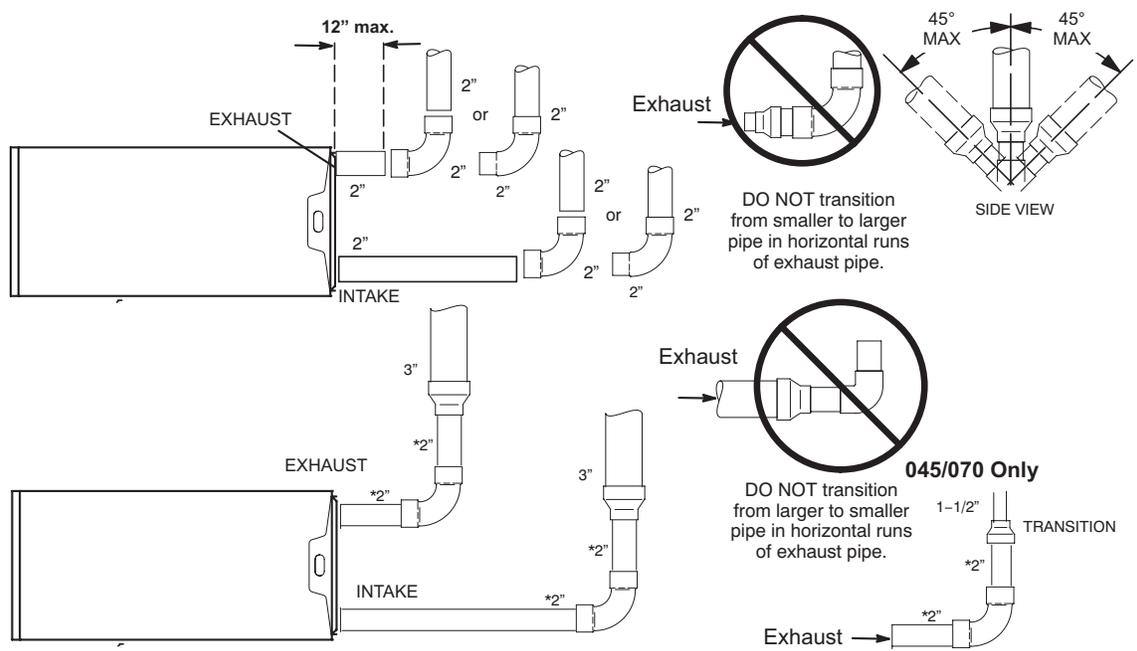
\* When transitioning up in pipe size, use the shortest length of 2" PVC pipe possible.
