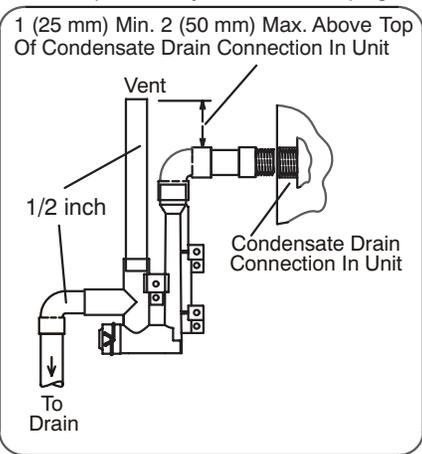
**Drain Trap Assembly with 3/4 inch Piping**
