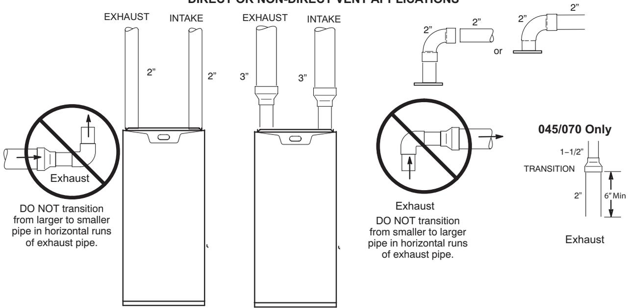
\* When transitioning up in pipe size, use the shortest length of 2" PVC pipe possible.
