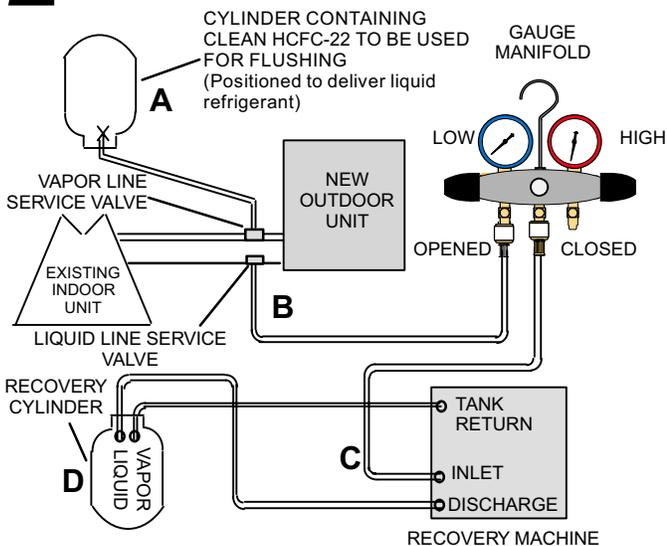
1. HCFC-22 cylinder with clean refrigerant (positioned to deliver liquid refrigerant) to the vapor service valve.
