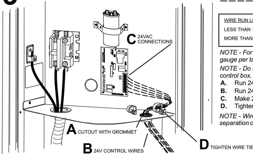
— HIGH VOLTAGE FIELD WIRING
