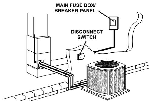
*NOTE - Units are approved for use only with copper conductors. Ground unit at disconnect switch or connect to an earth ground.*
