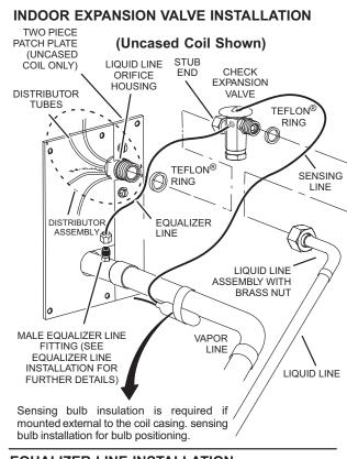
3 - Install one of the provided Teflon<sup>®</sup> rings around the stubbed end of the check expansion valve and lightly lubricate the connector threads and expose surface of the Teflon<sup>®</sup> ring with refrigerant oil.
