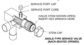
When service valve is **OPEN**, the service port is open to line set, indoor and outdoor unit.
