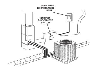
**NOTE -** Units are approved for use only with copper conductors. Ground unit at disconnect switch or connect to an earth ground.
