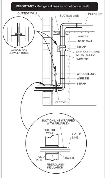
**NOTE** - Similar installation practices should be used if line set is to be installed on exterior of outside wall.
