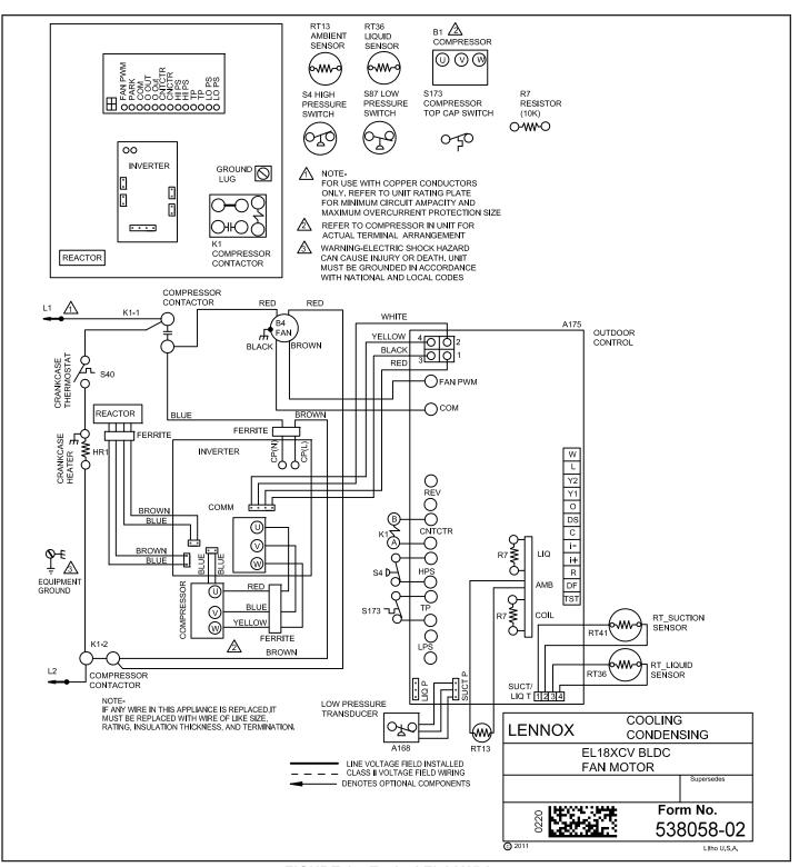
FIGURE 14. Typical Field Wiring
