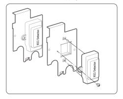
**3** Connect the wiring harness to the Refrigerant Detection Sensor socket and hang the wire on the wire-holder.
