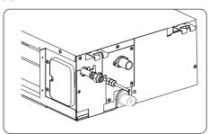
**2** Loosen 4 screws and remove the pipe cover, then remove the drain pump and cover .
