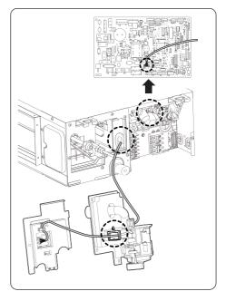
4 Reinstall the pipe cover, then reinstall the drain pump and drain cover.
