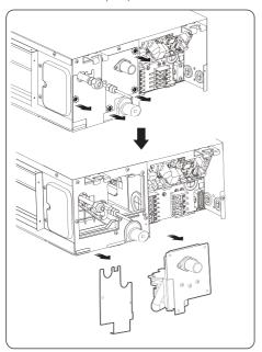
3 Connect the Refrigerant Detection Sensor wire with PBA through the wire-holder and Rubberhole.
