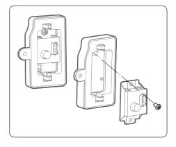
2 Attach the sensor and cover onto the piping cover with 1 of the self-tapping screws.
