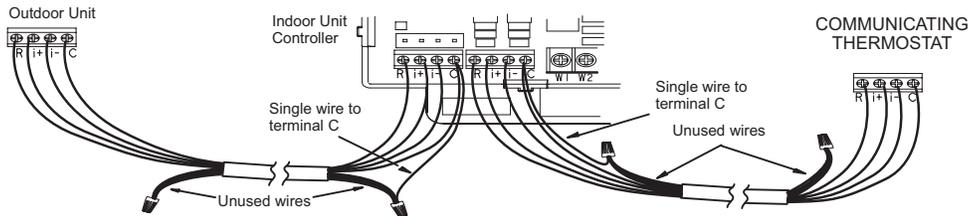
Communicating systems using the Communicating thermostat require four thermostat wires between the thermostat and the furnace/air handler control and four wires between the outdoor unit and the furnace/air handler control. When a thermostat cable with more than four wires is used, the extra wires must be properly connected to avoid electrical noise. The wires must not be left disconnected.
