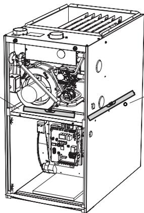
Place level on blower deck screws to check forward tilt
