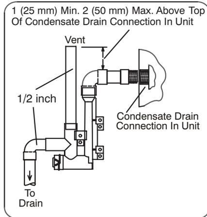
Drain Trap Assembly with 3/4 inch Piping
