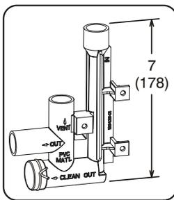
Drain Trap Assembly with 1/2 inch Piping
