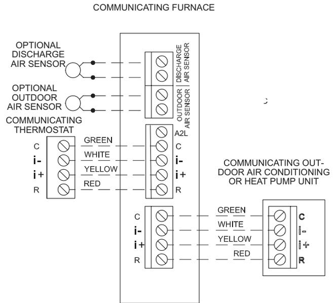
Communicating systems four thermostat wires between the thermostat and the furnace/air handler control and four wires between the outdoor unit and the furnace/air handler control. When a thermostat cable with more than four wires is used, the extra wires must be properly connected to avoid electrical noise. The wires must not be left disconnected.
