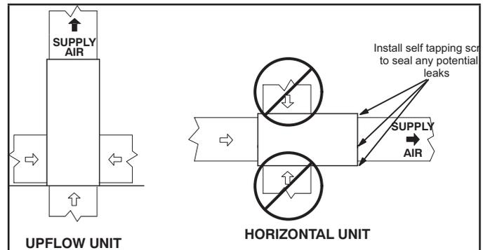
**NOTE** - Do not operate the furnace in the heating mode with an external static pressure that exceeds 0.8 inche w.c. Higher external static pressures may cause erratic limit operation.
