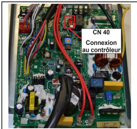
Figure 5. Circuit imprimé MCFA/B
