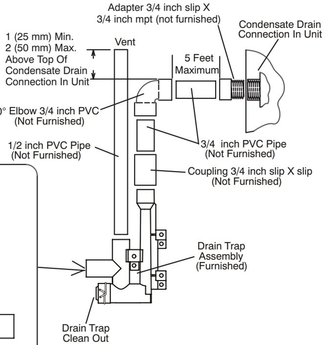
Drain Trap Assembly with 1/2 inch Piping
