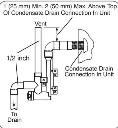
Drain Trap Assembly with 3/4 inch Piping
