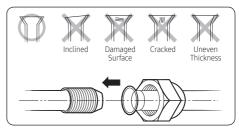
6 Align the pipes and tighten the flare nuts first manually and then with a torque wrench, applying the following torque.
