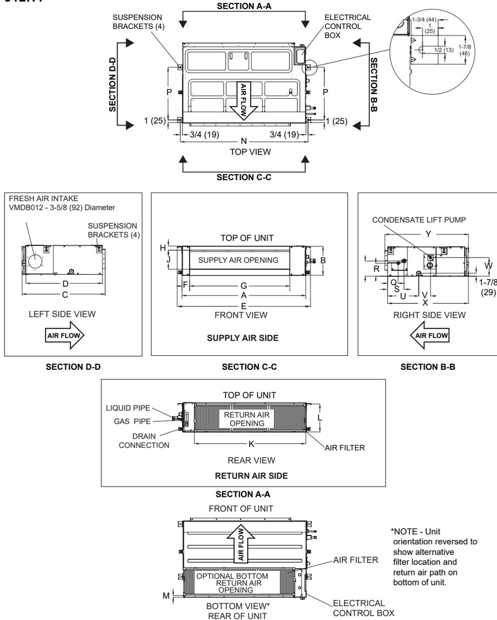
\*NOTE - Unit orientation reversed to show alternative filter location and return air path on bottom of unit.
