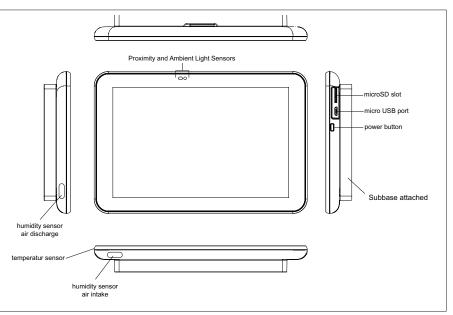
Figure 4. HD Display Components
