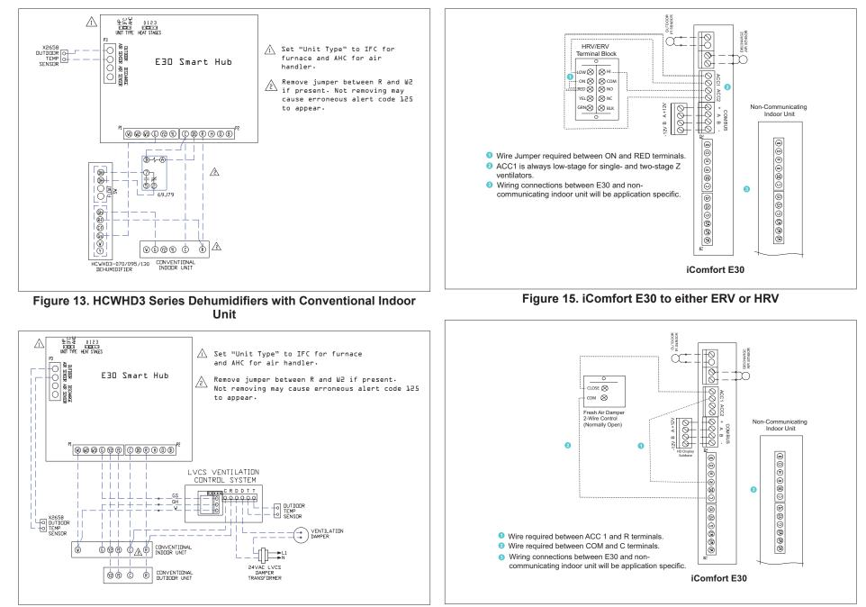
Figure 14. LVCS with Conventional Indoor and Outdoor Units
