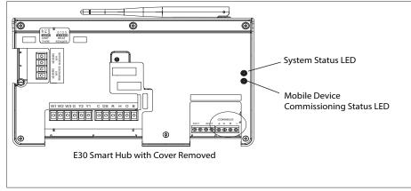
Figure 2. Smart Hub LED Indicators
