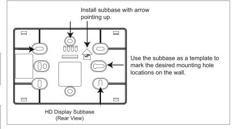
**9.** Drill 3/16" (5 mm) holes at marked locations on the wall for anchors. Then insert wall anchors into holes until flush with the wall.
