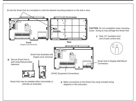
Figure 17. Smart Hub Installation
