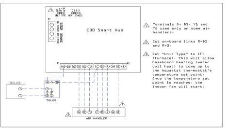
Figure 10. Hydronic Baseboard Heating with Conventional Air Handler
